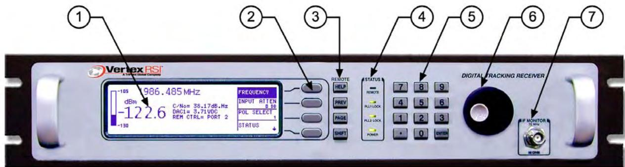
Figure 1-1 DTR Front Panel
