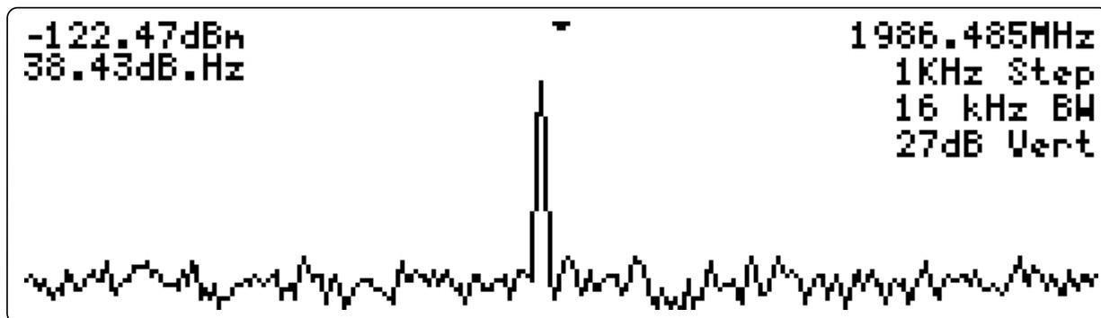
Figure 4-3 Spectral Display
