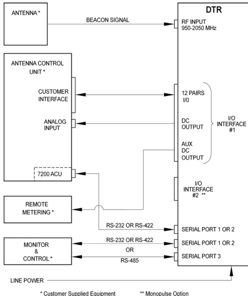
Figure 3-1 L-Band DTR-I/O Connections
