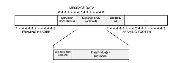
In this protocol, the first byte of the message data is referred to as the *instruction code*, which ranges in value from **00** to **20**. Normally if there is a reply, it will contain the same instruction code as the host message.
