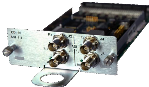
Figure 10-3. ASI Interface (PL/10881-4) For 1:1 Applications
