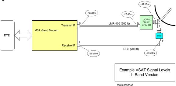
There is virtually no control over the receive signal levels short of setting the antenna size. The demodulator uses a sliding AGC window with an approximate AGC range of 55 dB at any given data rate. As the data rate is decreased the AGC window moves down to accommodate the decreasing signal level.
