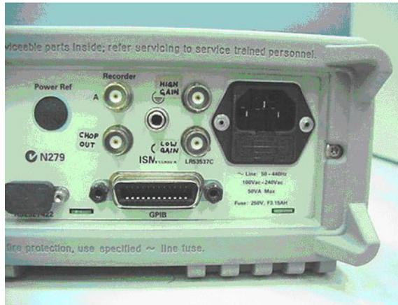
**Figure A-11** Label the BNC connectors with a permanent marker and adhesive labels
