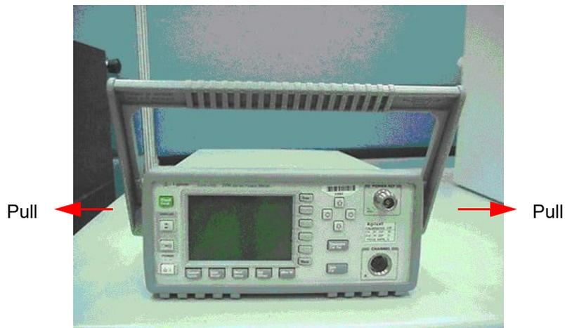
**Figure A-2** Remove the power meter handle
