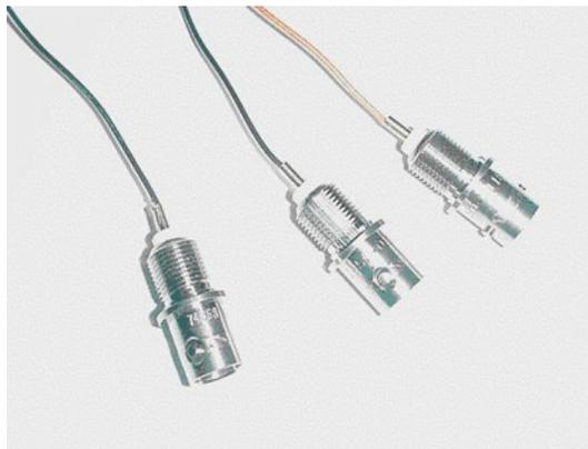
**Figure A-7** Solder each wire onto the screw-fit BNC female connectors
