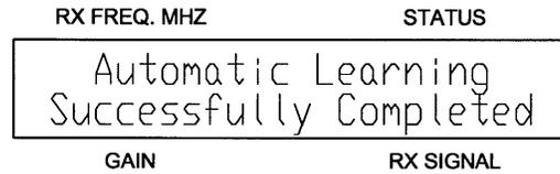
**Figure 4-15. Automatic Learning Successfully Completed Window**
