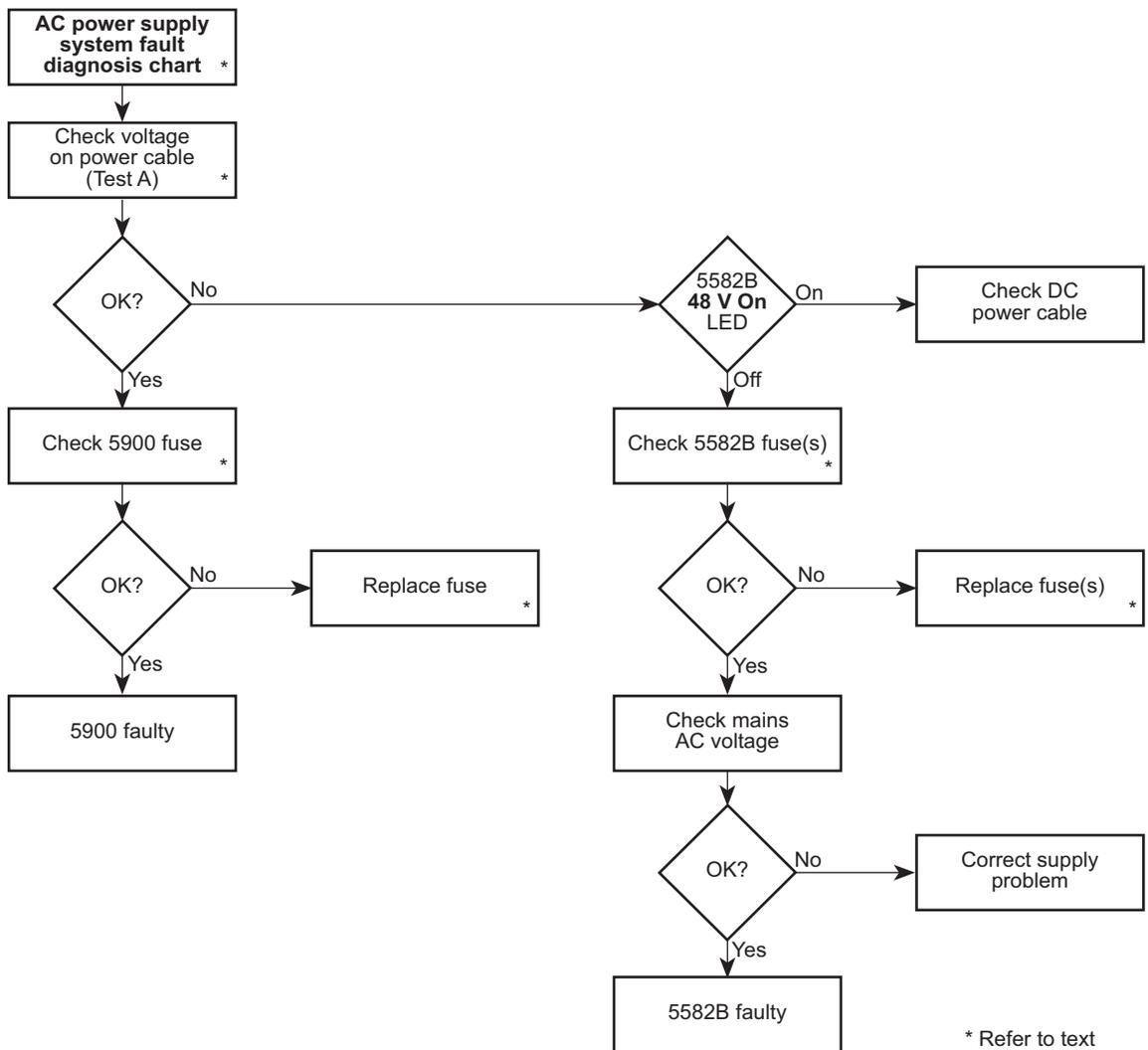
Figure 9-6: 5940 SSPA supply system fault diagnosis chart
