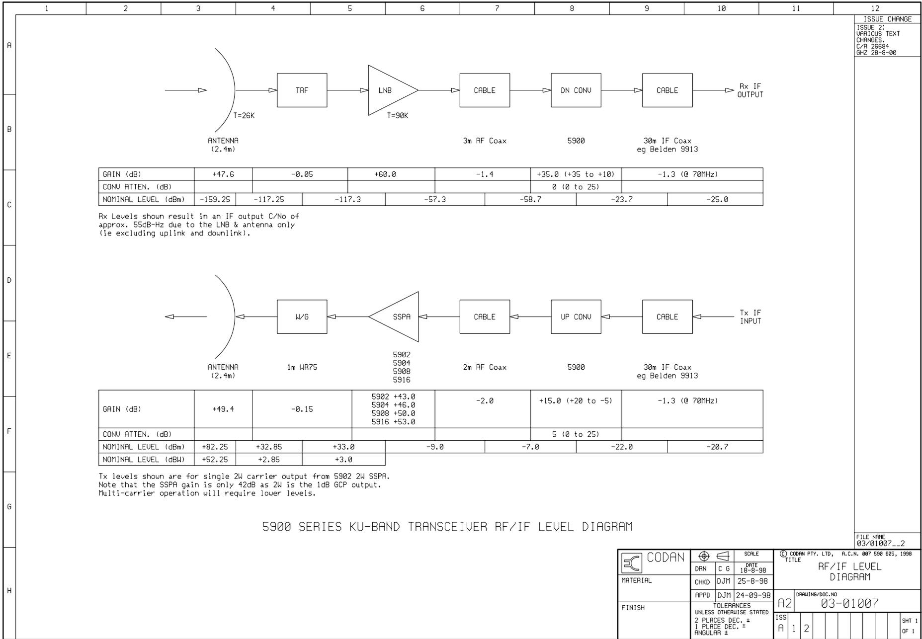
5900 SERIES KU-BAND TRANSCEIVER RF/IF LEVEL DIAGRAM
