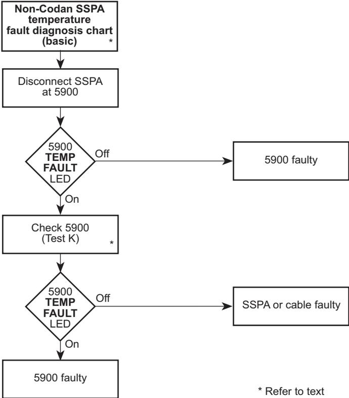
Figure 9-13: Temperature fault diagnosis chart for a basic interface (5940 SSPA)
