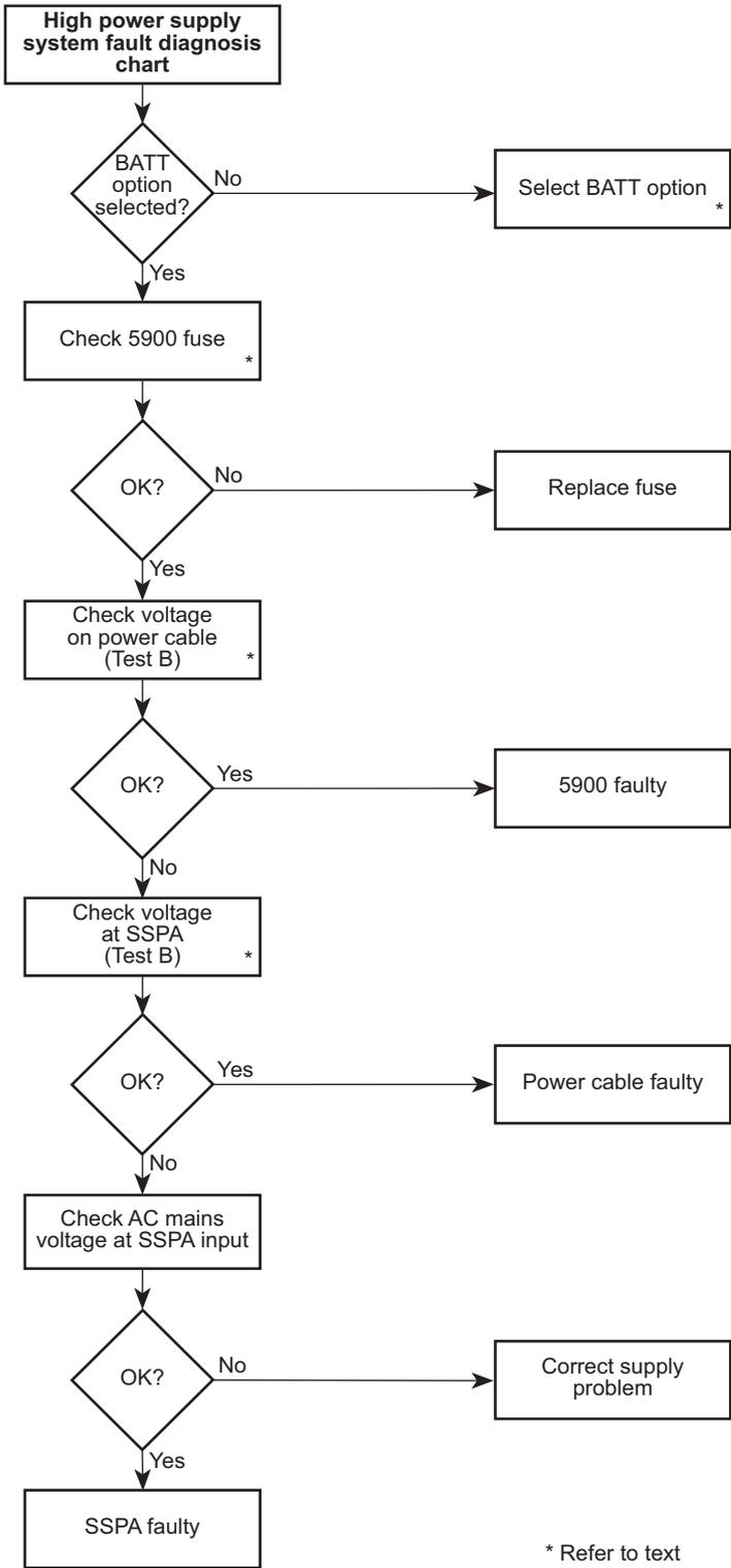
Figure 9-7: 5904/5908/5916 SSPA fault diagnosis chart for an extended interface
