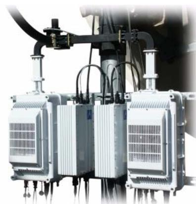
Redundant C-Band 60 W high power transceiver system
