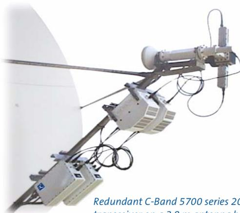
Redundant C-Band 5700 series 20 W transceiver on a 3.8 m antenna boom
