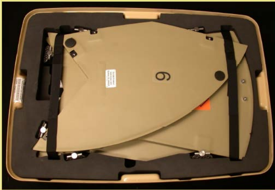
Figure 3 Backpack A - Antenna/RF Lid with Antenna Segments
