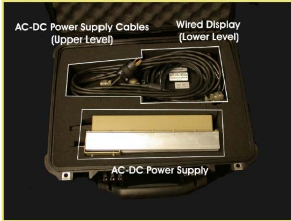
Figure 7 Transit Case C - AC-DC Power Supply and Wired Display (optional)
