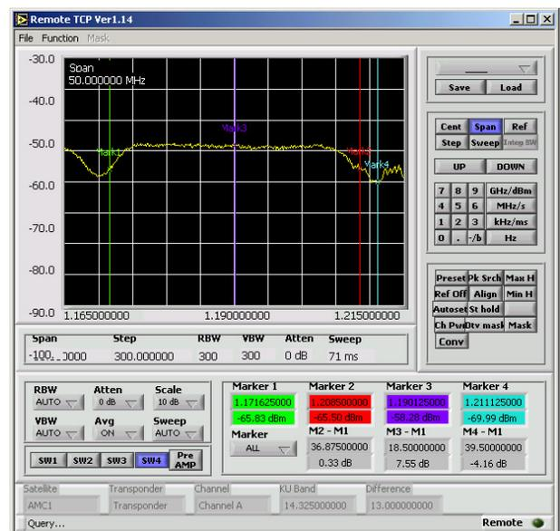
Figure 1: A Typical Carrier Measurement
