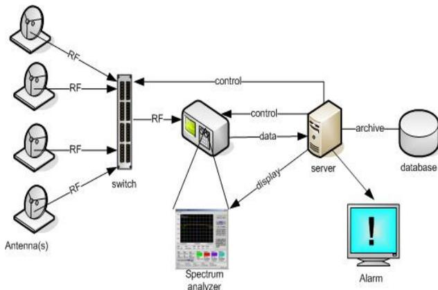
Figure 2: Basic Spectrum Monitor System
