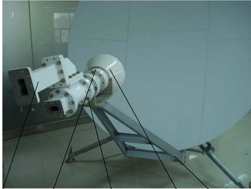
1 The reflector bracket 2 Semicircle Clasp 3 Transition Chassis 4 The feed 5 The feed bracket
