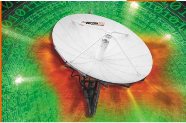
The VertexRSI 4.8-Meter C, X, and Ku-band antenna delivers exceptional performance for receive-only and for transmit/ receive applications world-wide. Model 4.8 KPC/KPX/KPK Compact Cassegrain antennas feature all metal reflectors which incorporate doubly-contoured, formed panels with matched radials and hub assemblies for easy bolt-together installation with no field alignment required.
