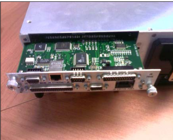
Removable rear panel monitor and control card
