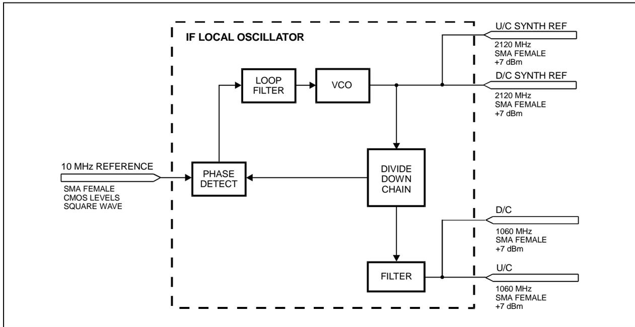
**Figure 6-5. IF Local Oscillator Block Diagram**
