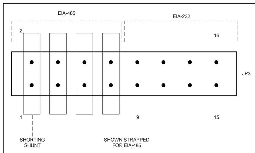
**Figure 6-2. M&C Jumper Placement at JP3**
