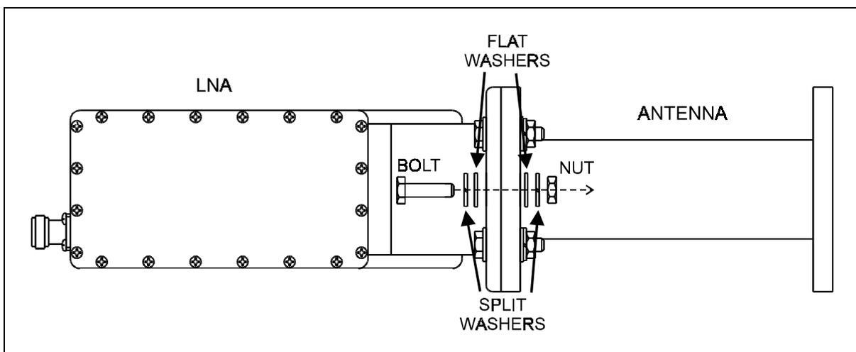
**Figure 3-2. Installation of the LNA**
