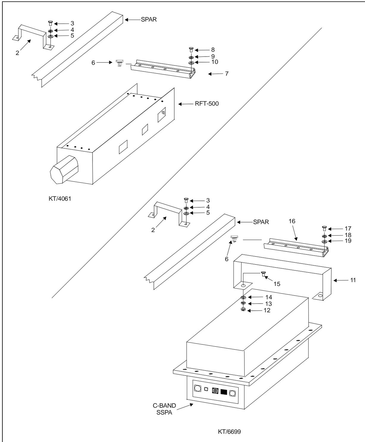
Figure 8-3. Exploded View of Spar Mounting Kit (Single Thread Configuration)
