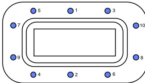
**Figure 3-3. Procedures for Tightening the Waveguide Bolts**
