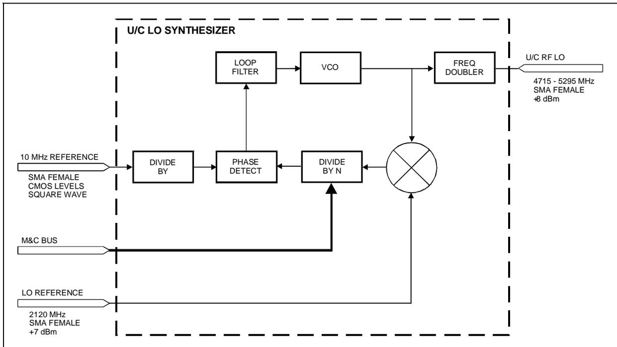
Figure 6-7. Up Converter Synthesizer Block Diagram
