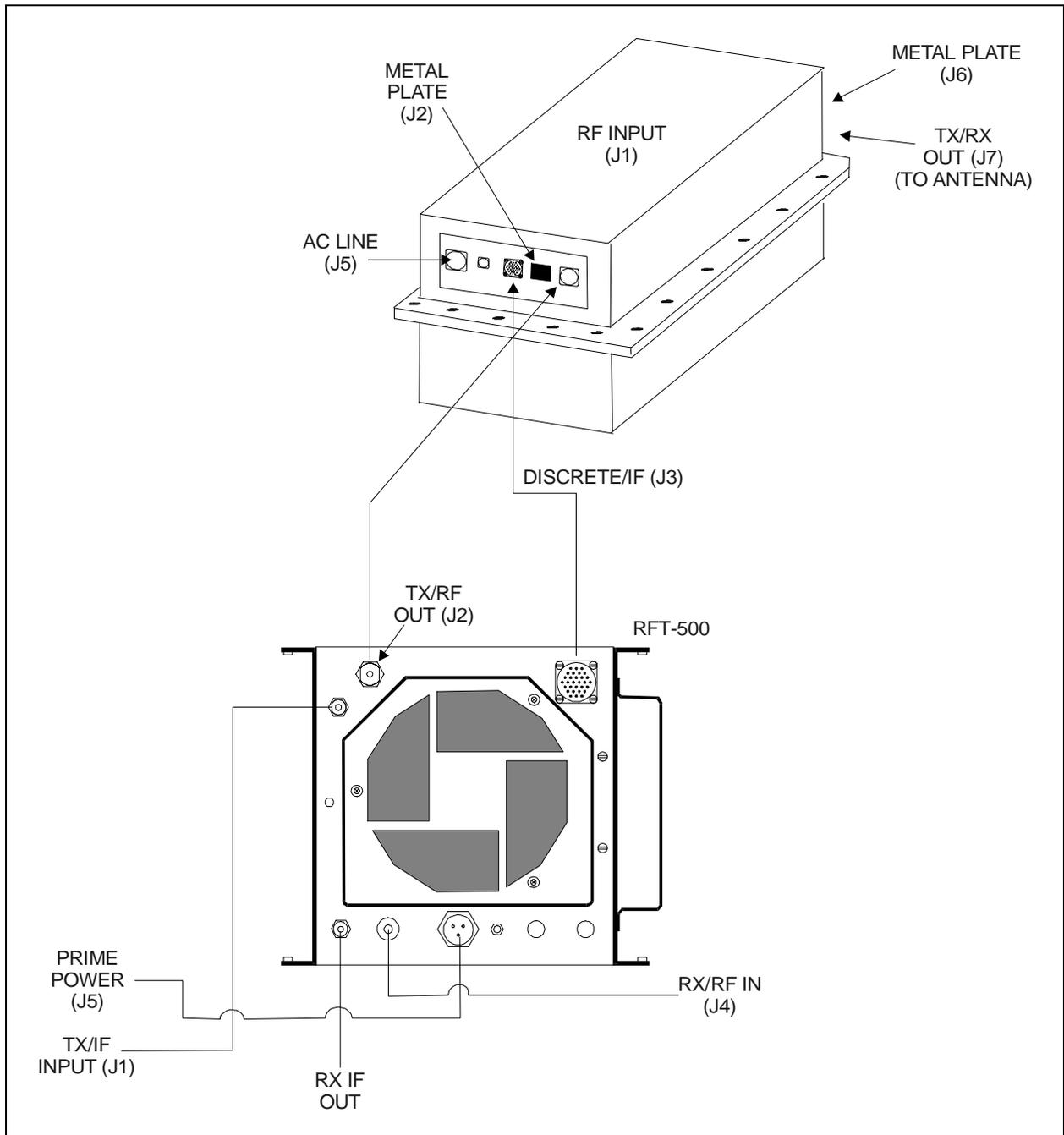
**Figure 3-1. HPCST-5000 Single Thread Configuration Schematic**
