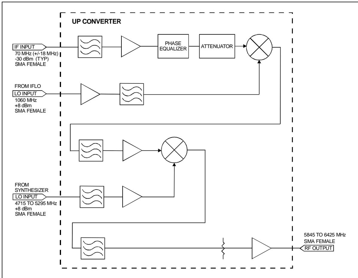
Figure 6-9. Up Converter Block Diagram
