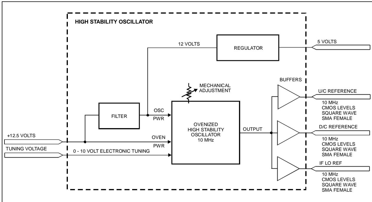
**Figure 6-4. High Stability Oscillator Block Diagram**
