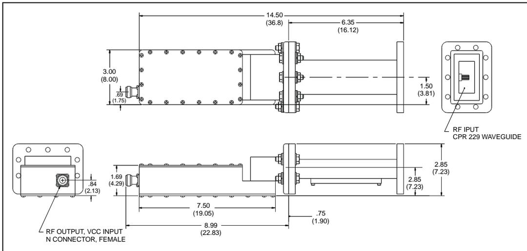
**Figure 1-9. Single Thread Configuration Dimensional Requirements**
