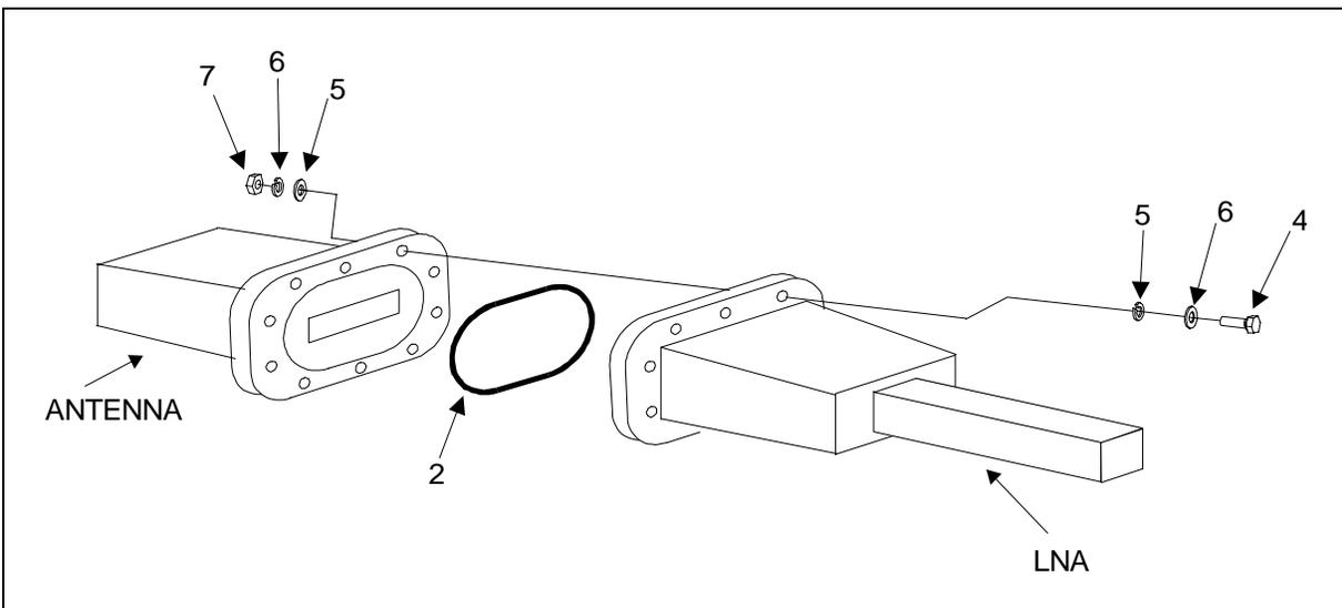
**Figure 8-1. Exploded View of a Typical LNA Connector Kit**
