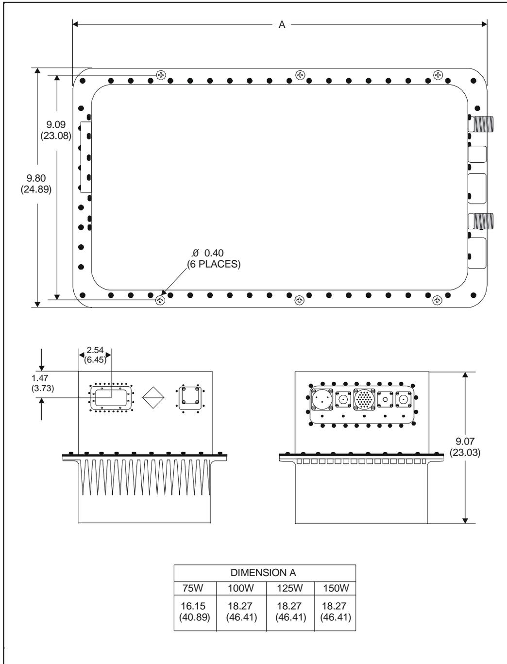
**Figure 1-8. C-Band SSPA Dimensional Requirements**
