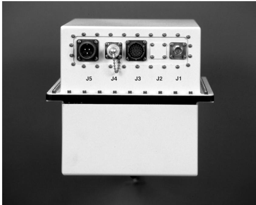
**Figure 2-3. C-Band SSPA External Connections**
