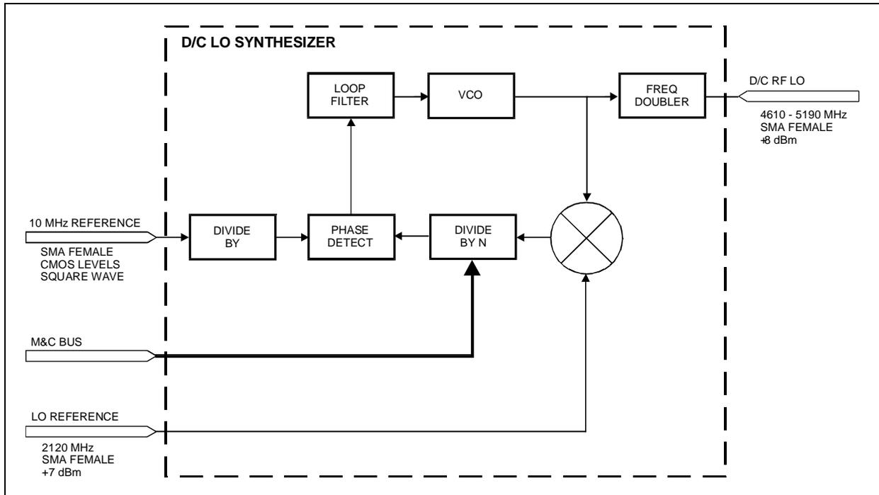
Figure 6-6. Down Converter Synthesizer Block Diagram
