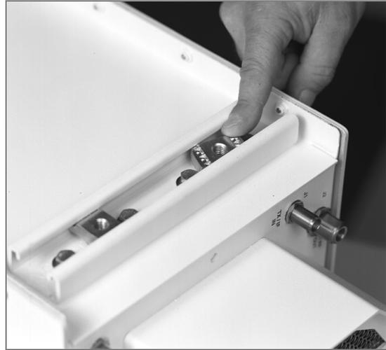
(2) Press down on the spring nut to compress the spring, and rotate the nut 90° (i.e., perpendicular to the unistrut).
