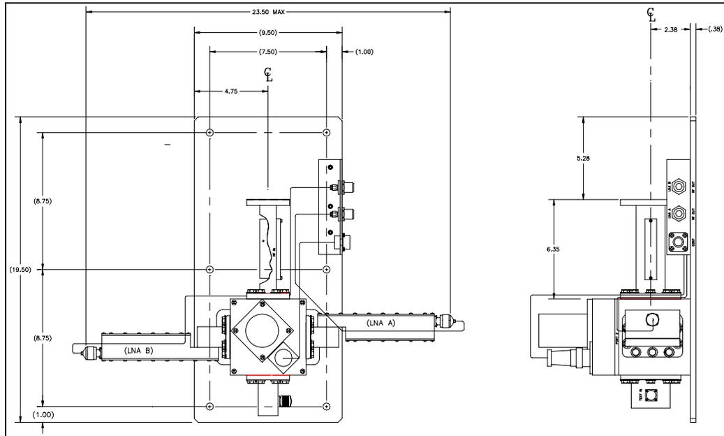
**Figure 1-10. Standard Redundant Configuration Dimensional Requirements**
