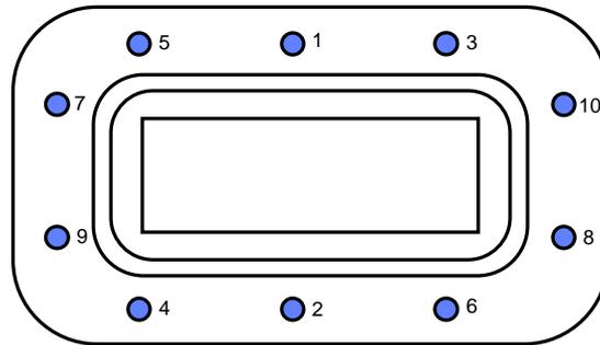
**Figure 4-4. Procedures for Tightening LNA to Waveguide Bolts**
