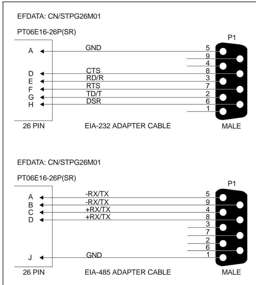
**Figure 2-2. Serial Adapter Cables**
