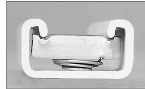
(2) Press down on the spring nut to compress the spring, and rotate the nut 90° (i.e., perpendicular to the unistrut).
