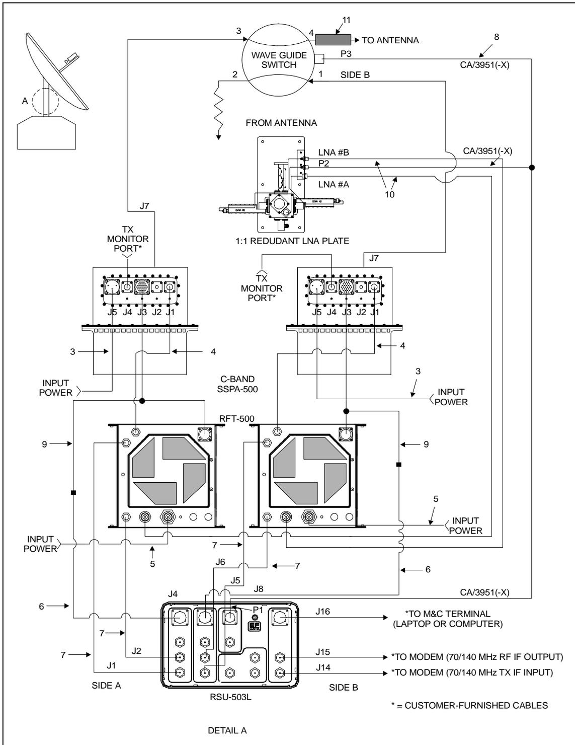
Figure 8-2. 1:1 Redundant Configuration Cabling
