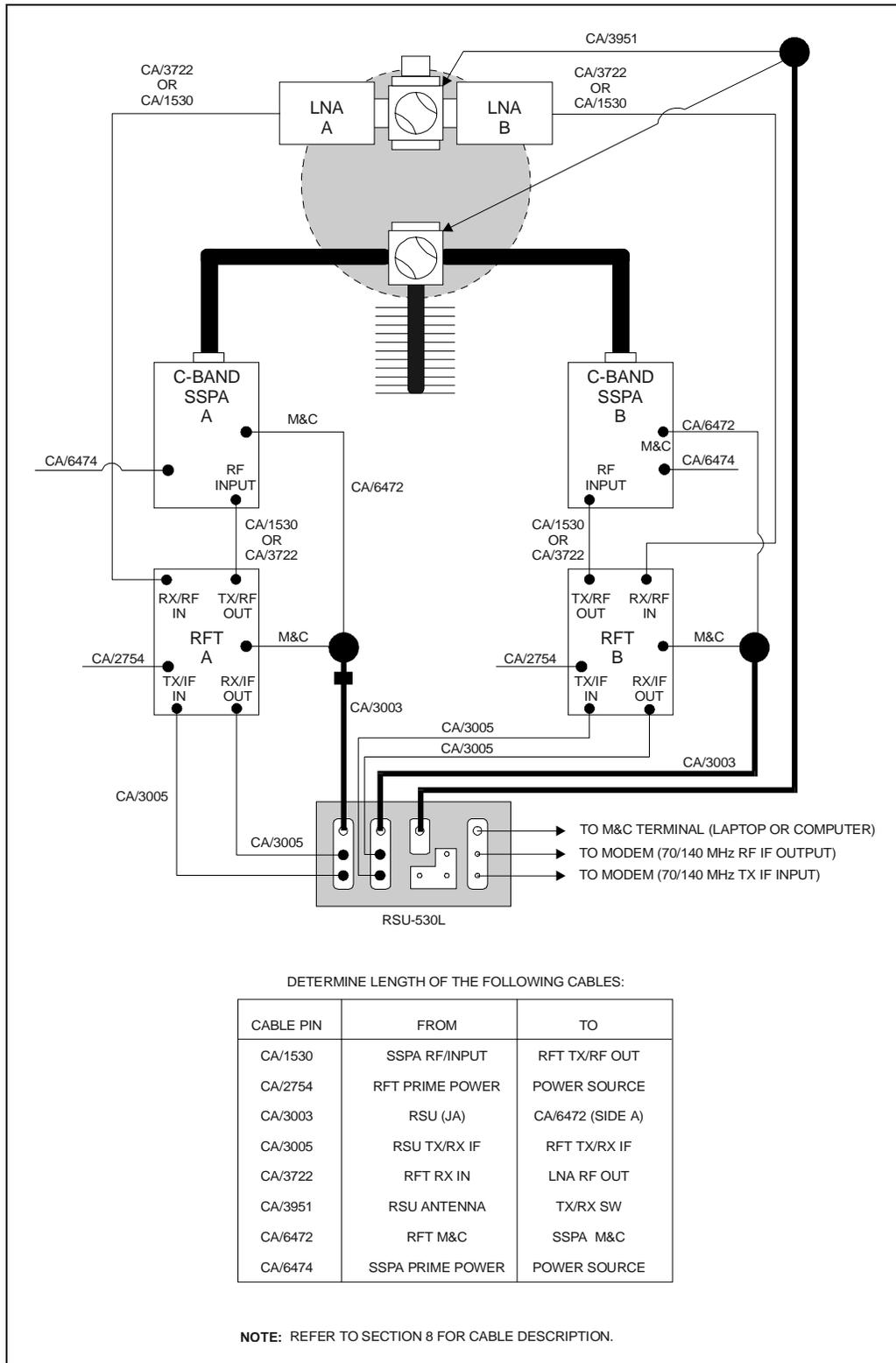
**Figure 4-5. Redundant Configuration Cable Assembly Matrix**
