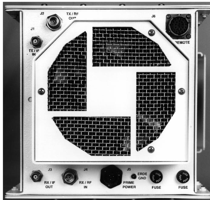
**Figure 2-1. RFT External Connections**
