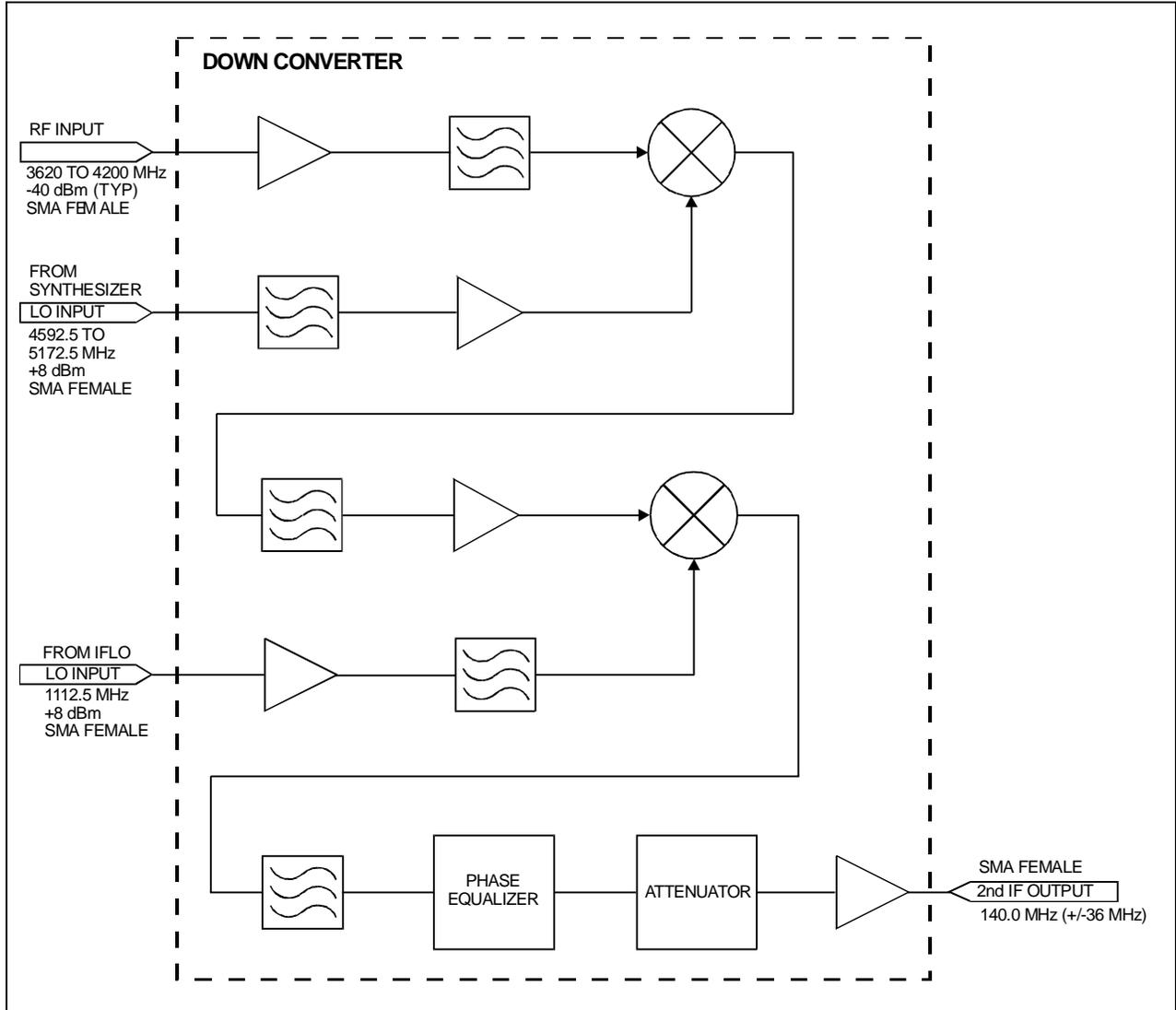
Figure A-4. Down Converter Block Diagram
