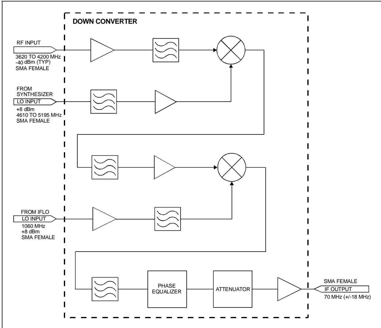
Figure 6-8. Down Converter Block Diagram
