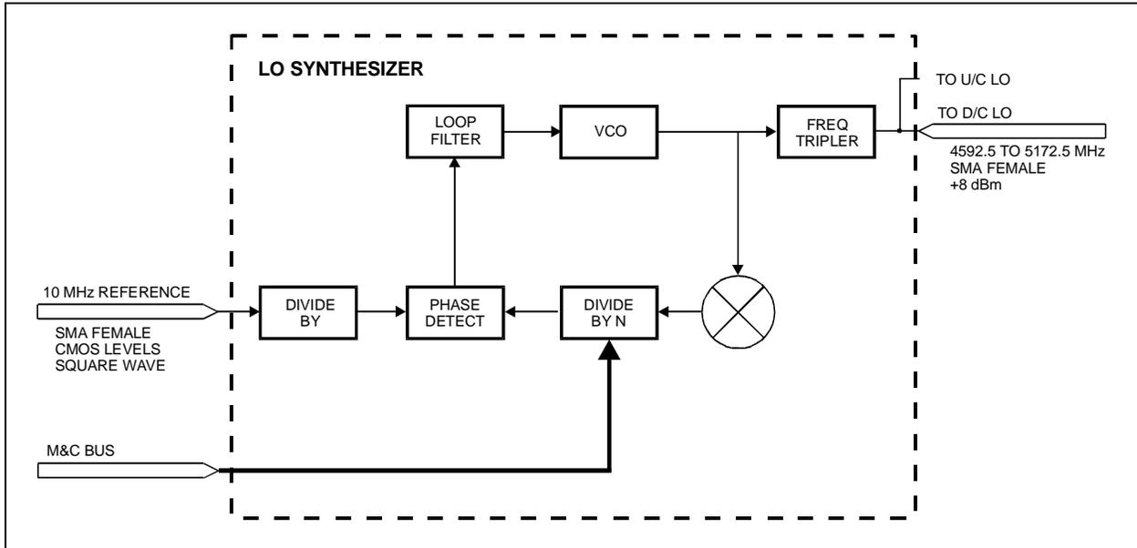
Figure A-2. LO Synthesizer Block Diagram
