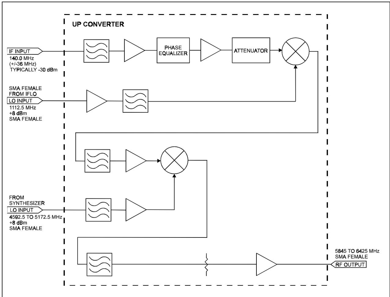
Figure A-5. Up Converter Block Diagram
