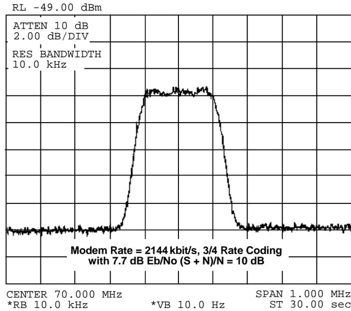
Figure A-2. Typical Output Spectrum – With Noise
