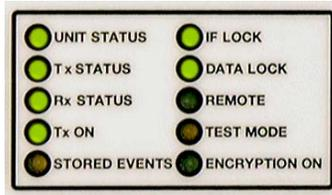
The ten LEDs located on the modem's front panel indicate status, fault, and alarm information.
