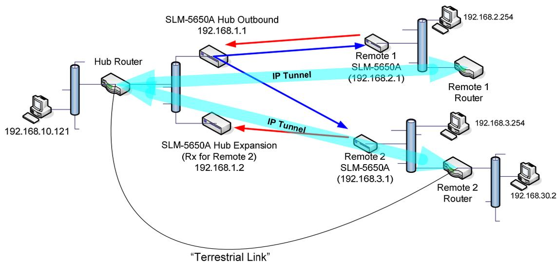
Figure E-5. OSPF Test Solution
