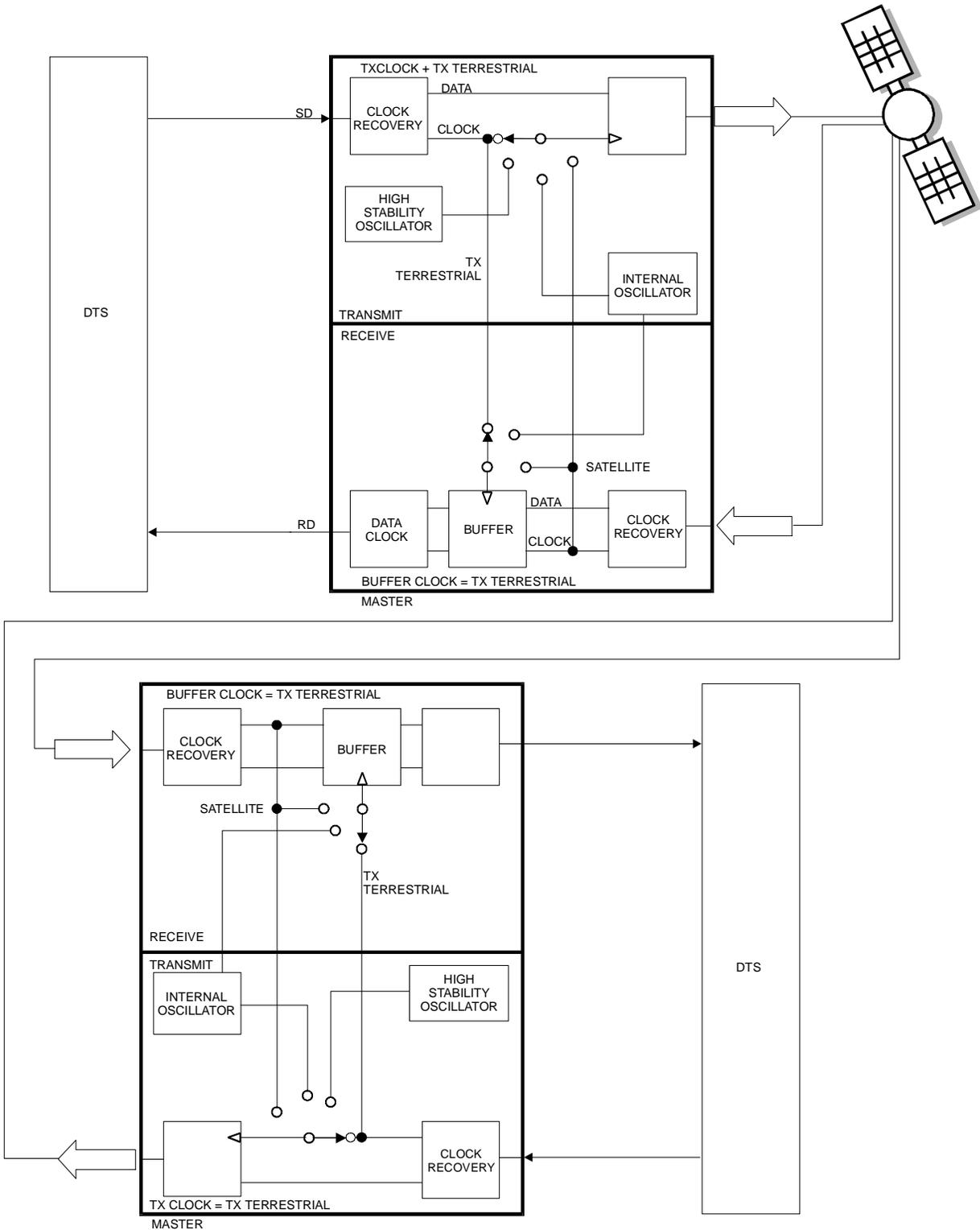
Figure B-1. IDR/IBS G.703 Master/Master Clocking Diagram
