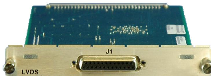
**Figure 13-1. Low Voltage Differential (LVDS) Interface Module (PL/12272-1)**
