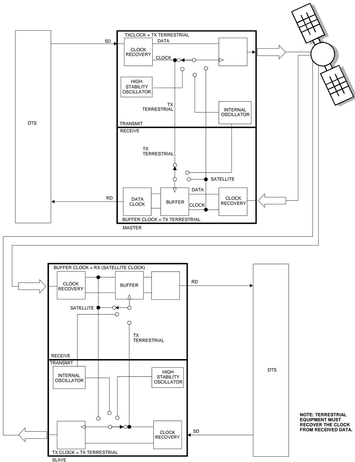
Figure B-2. IDR/IBS G.703 Master/Slave Clocking Diagram
