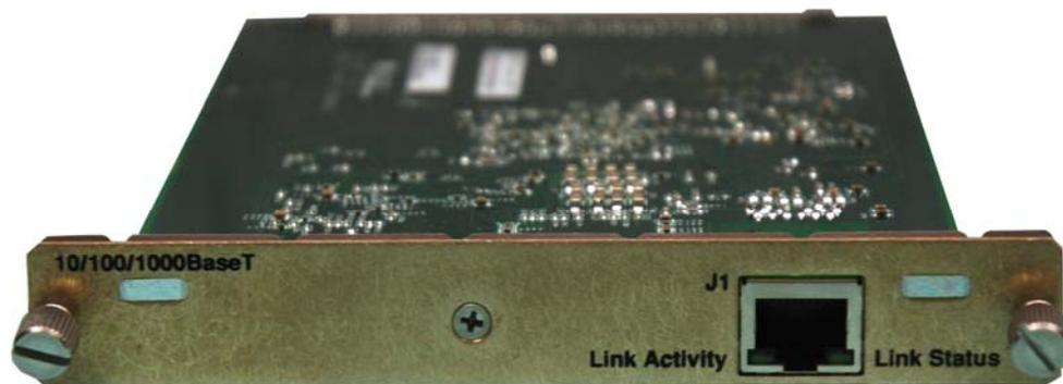
**Figure 11-1. 10/100/1000 Base-T (GbE) Interface Module (AS/11985)**
