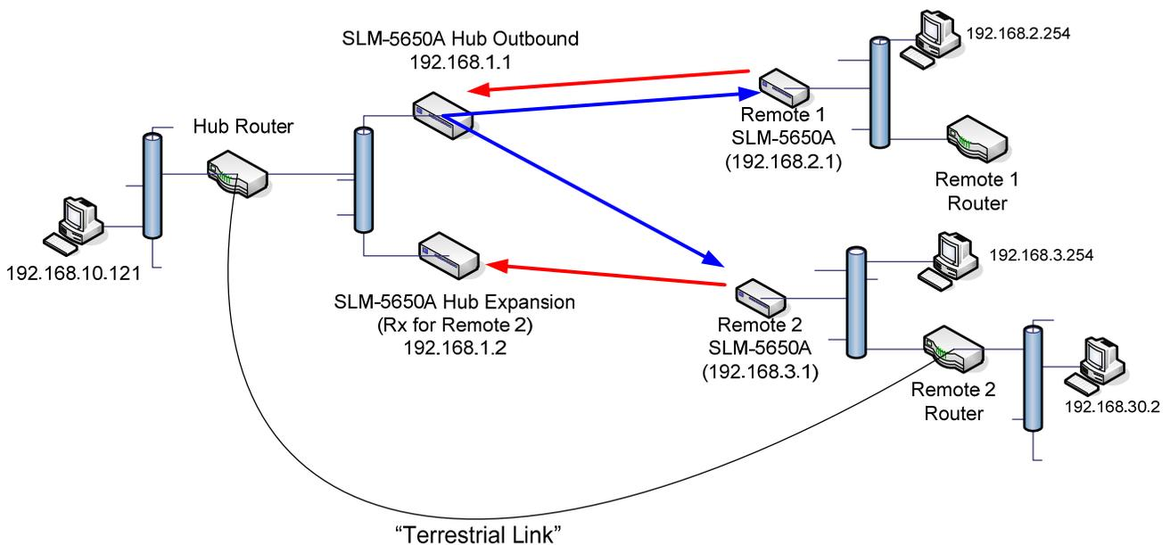
**Figure E-4. OSPF Laboratory Test Network**
