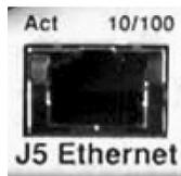
The J5 Ethernet connection is an 8-pin 'RJ-45' type 10/100 Base-T connector. Remote control of the modem is provided using SNMP, HTTP or Telnet with this port.
