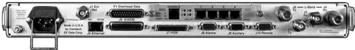
**Figure 3-1. SLM-5650A Rear Panel (with optional Network Processor Interface installed)**
