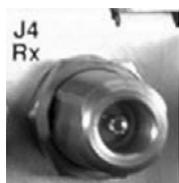
The L-Band IF Interfaces use standard 50  $\Omega$  Type 'N' female connectors.
