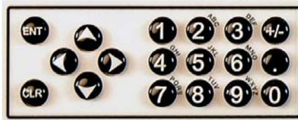
The front panel keypad controls the local operation of the modem. The keypad consists of 18 keys. Each key provides one or more logical functions.
