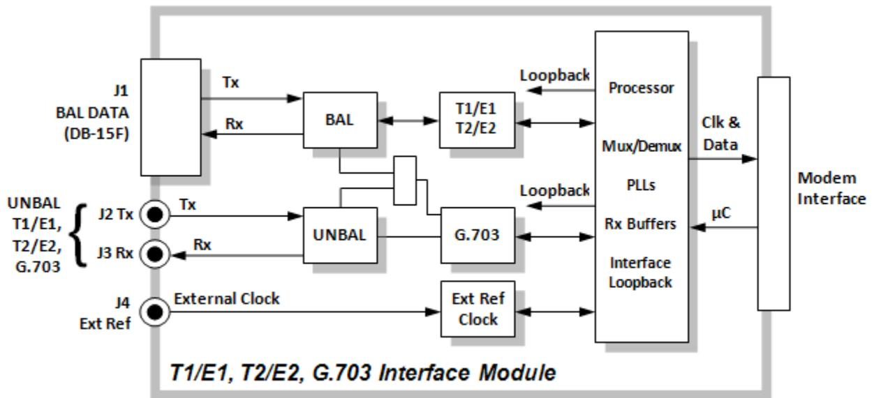
Figure 12-2. T1/E1, T2/E2, G.703 Interface Functional Block Diagram
