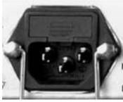
A standard, detachable, non-locking, 3-prong power cord (IEC plug) supplies the Alternating Current (AC) power to the modem. Observe the following:
