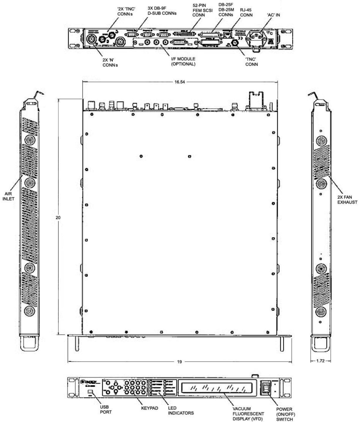
Figure 1-3. SLM-5650A Dimensional Envelope
