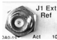
The J1 external reference uses a standard 50  $\Omega$  TNC female connector.
