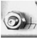
A #10-32 stud on the rear panel of the modem is used for connecting a common chassis ground among all equipment.
