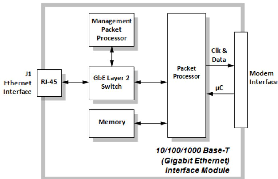
Figure 11-2. GbE Interface Functional Block Diagram
