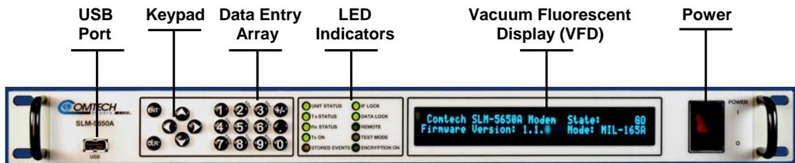
**Figure 5-1. Modem Front Panel**
