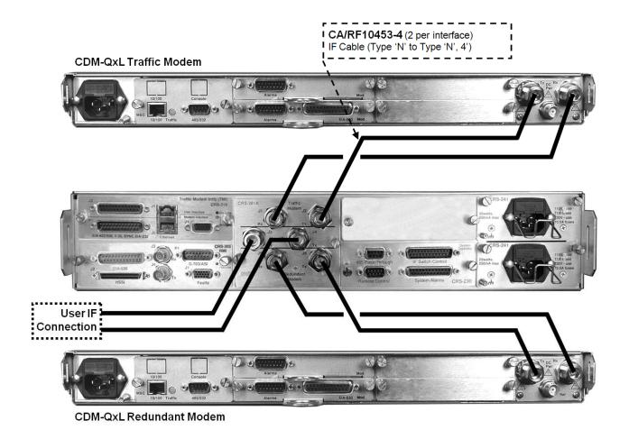
Figure 3-8. CDM-QxL IF Cabling Example – CRS-281A (L-Band)
