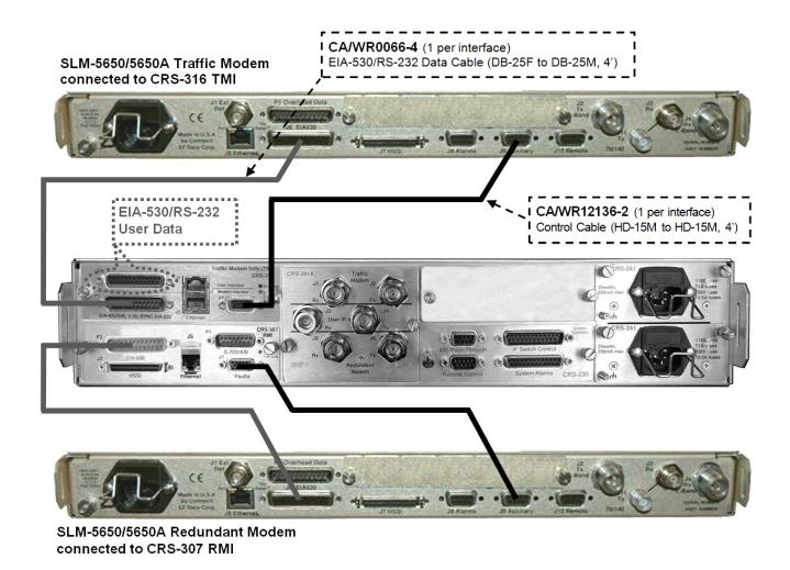
Figure 3-11. SLM-5650/5650A Control and EIA-530 Traffic Data Cables
