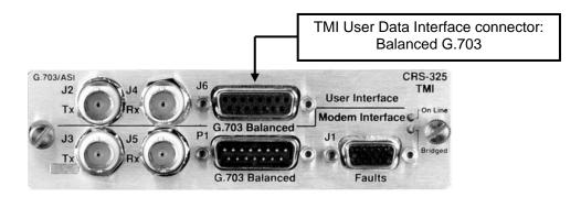
**Table 5-5** indicates the pinout for the DB-15F Balanced G.703 User Data Interface connector: "J6" on the CRS-325 TMI.
