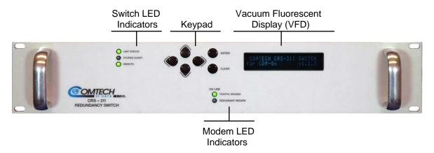
Figure 6-1. CRS-311 Front Panel
