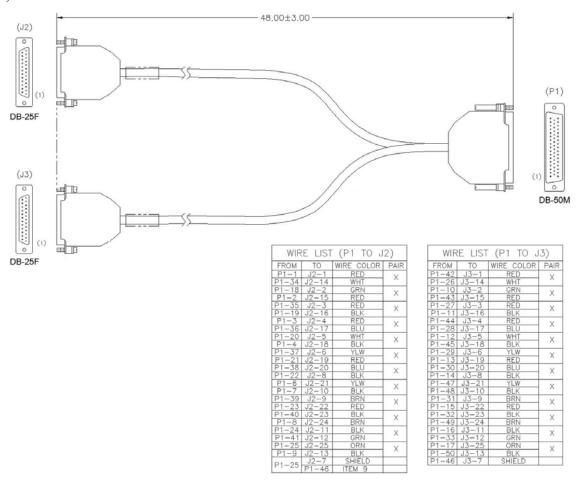
Figure A-10. SLM-5650/5650A Control 'Y' Overhead Cable (CA-0000006)
