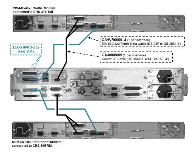
Figure 3-2. CDM-Qx/QxL Control 'Y' and EIA-530/RS-232 Traffic Data Cables
