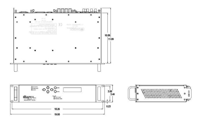
Figure 1-22. CRS-311 Dimensional Envelope
