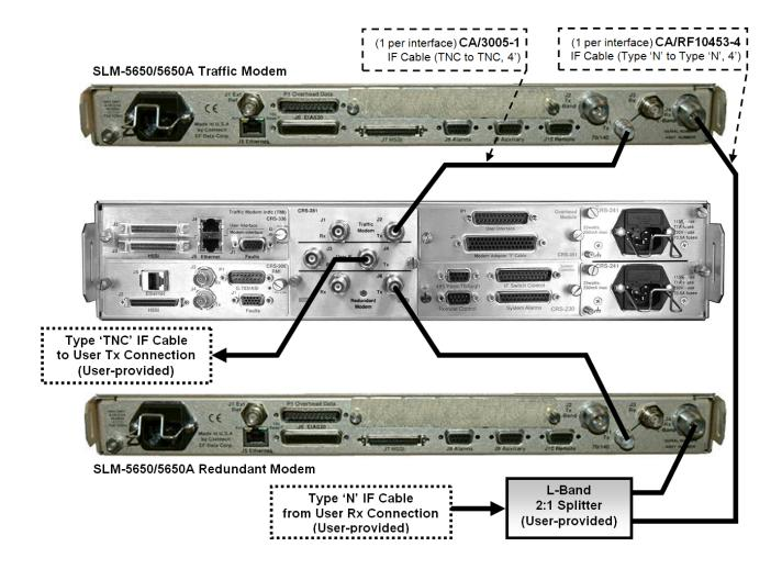
Figure 3-18. SLM-5650/5650A Mixed IF Band Cabling Example – CRS-281L (70/140 MHz Tx, L-Band Rx)
