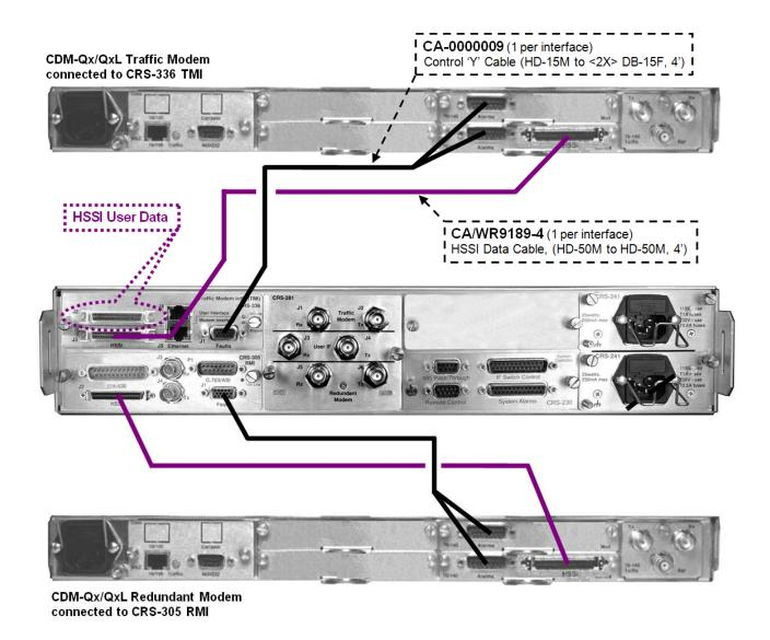
Figure 3-5. CDM-Qx/QxL Control and HSSI Traffic Data Cables
