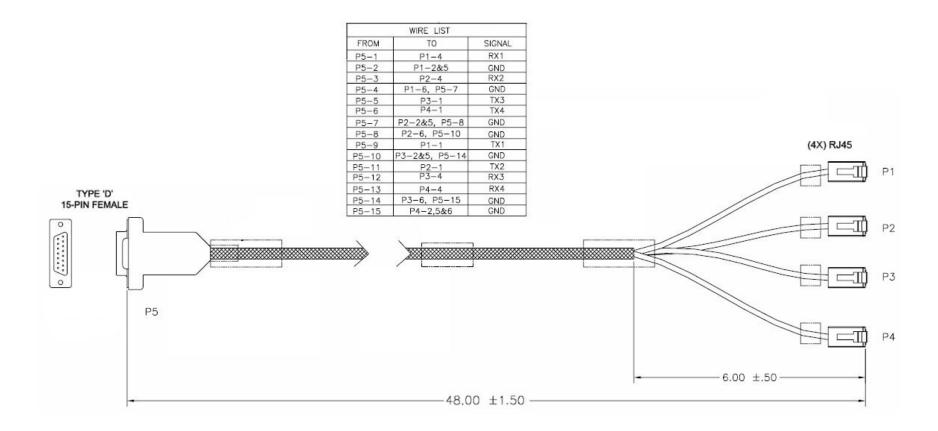
Figure A-16. CDM-Qx/QxL Quad E1 Data Cable (CA/WR13018-2)
