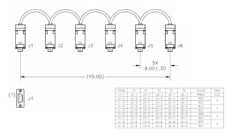
Figure A-5. Standard RS-485 Multi-Drop Shielded Cable (CA-0000096)
