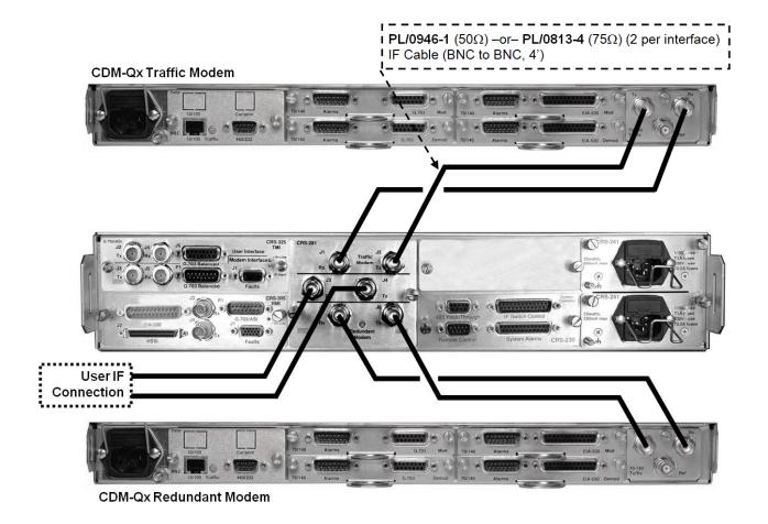
Figure 3-7. CDM-Qx IF Cabling Example – CRS-281 (70/140 MhZ,  $50\Omega$  or  $75\Omega$  BNC)
