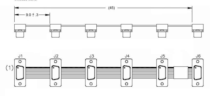
Figure A-4. Optional RS-485 Multi-Drop Ribbon Cable (CA-0000095)
