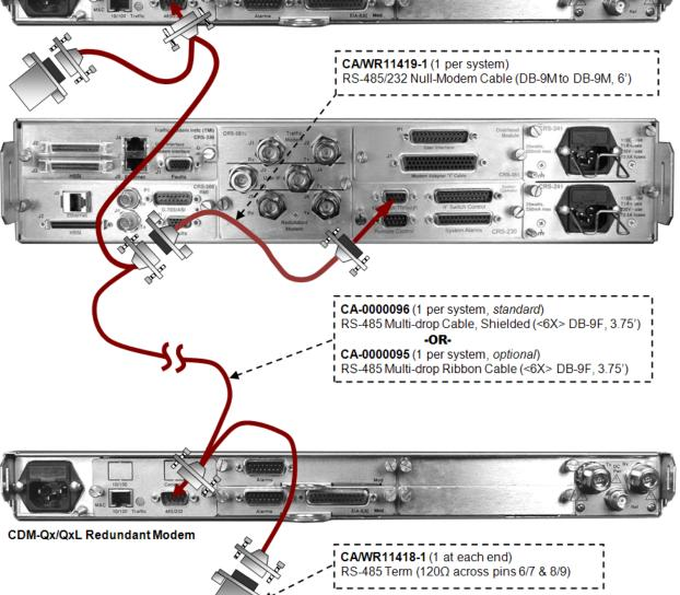
Figure 3-1. CDM-Qx/QxL Cabling Example – RS-485 Multi-drop Cable
