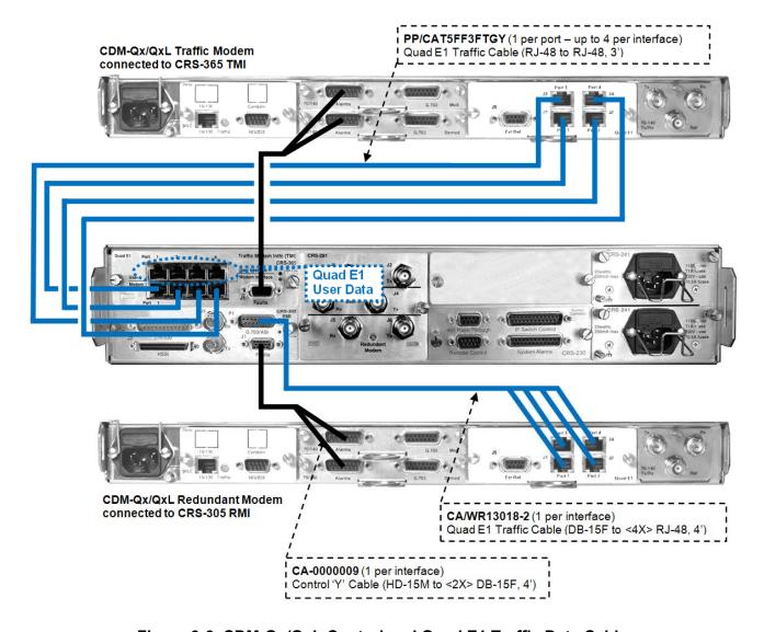
Figure 3-6. CDM-Qx/QxL Control and Quad E1 Traffic Data Cables
