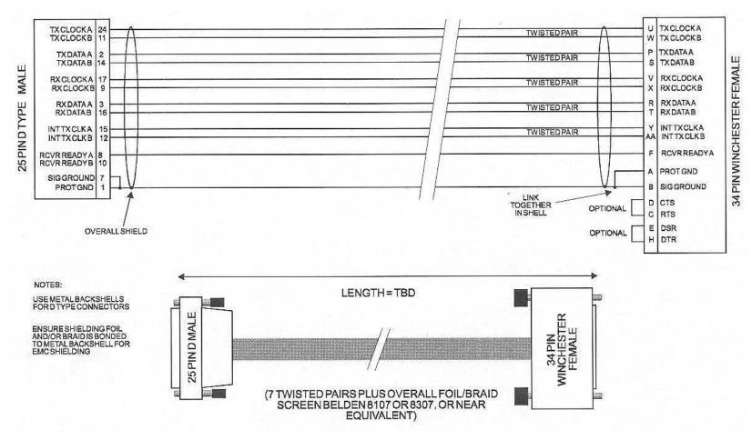
Figure A-2. DCE Conversion Cable: RS-530 to V.35
