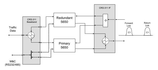
Figure D-1. Standard Connections to CRS-311
