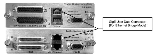
**Table 5-8** indicates the pinout for the RJ-45F TMI User Data Interface connector (Gigabit Ethernet): "J4" on the CRS-316 and the CRS-336 TMIs.
