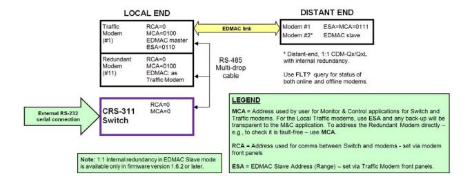
Figure B-3. CRS-311 Addressing Scheme Example: External RS-232 with CDM-Qx/QxL Modems
