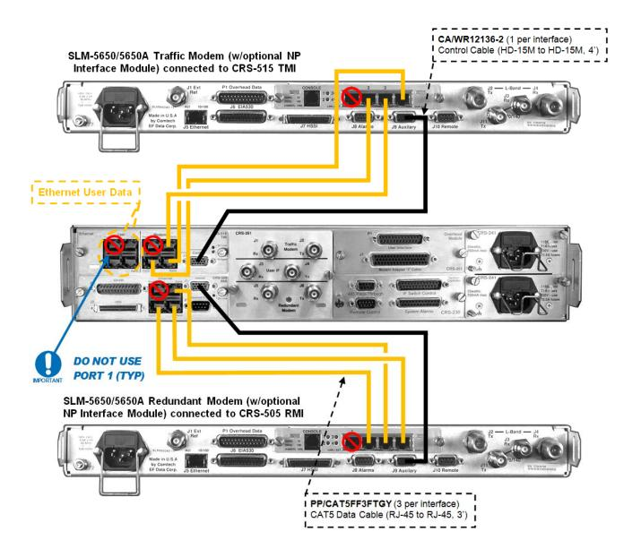
Figure 3-12. SLM-5650/5650A Control and Ethernet Traffic (Multi-Port Bridge Mode)
