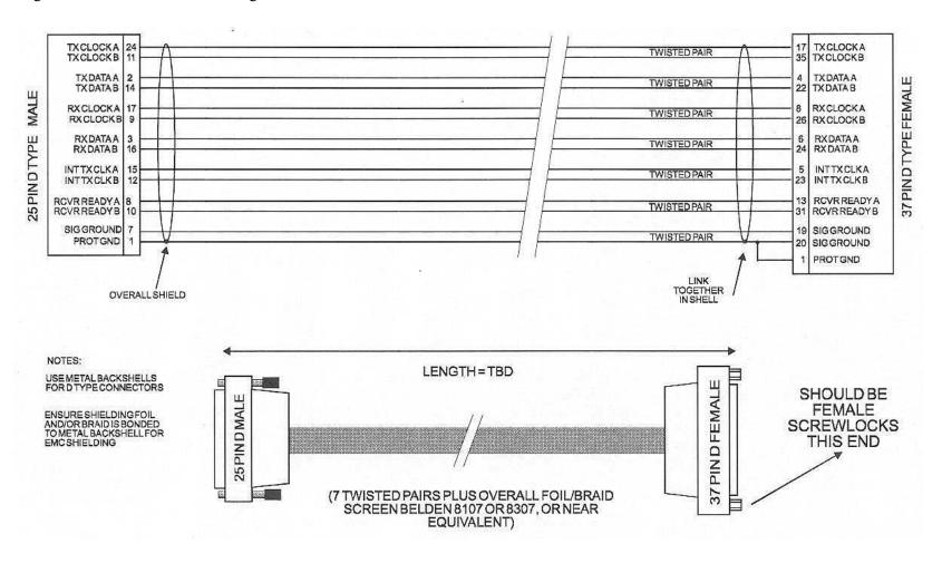
Figure A-1. DCE Conversion Cable: RS-530 to RS-422/449
