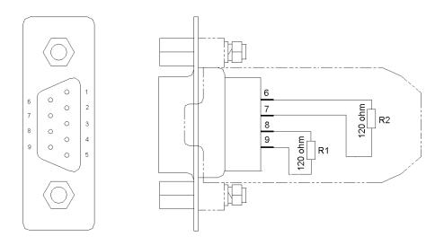
Figure A-6. RS-485 Cable Termination (CA/WR11418-1)
