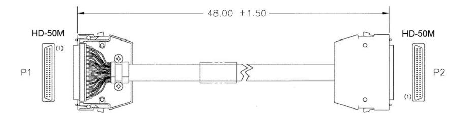
Figure A-15. HSSI Data Cable (CA/WR9189-4)
