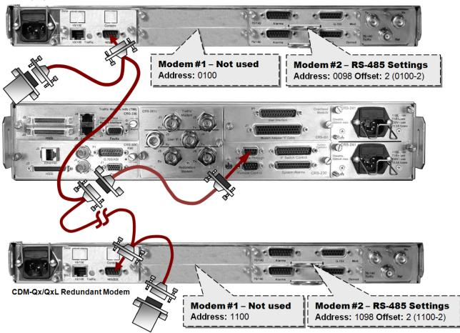
Figure 4-2. CDM-Qx/QxL / CRS-311 RS-485 Scheme
