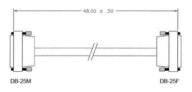
Figure A-12. RS-232/422, EIA-530 Control and Data Cable (CA/WR0066-4)
