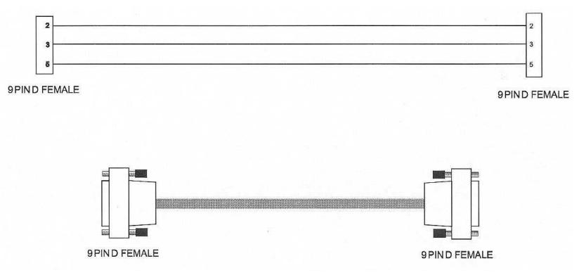
Figure A-3. Switch Programming Cable
