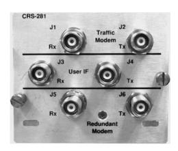
Figure 1-17. CRS-281 IF Switch Module: 70/140 MHz Type 'BNC' (PL/12040-3 [75 $\Omega$ ] or PL/12040-4 [50 $\Omega$ ])
