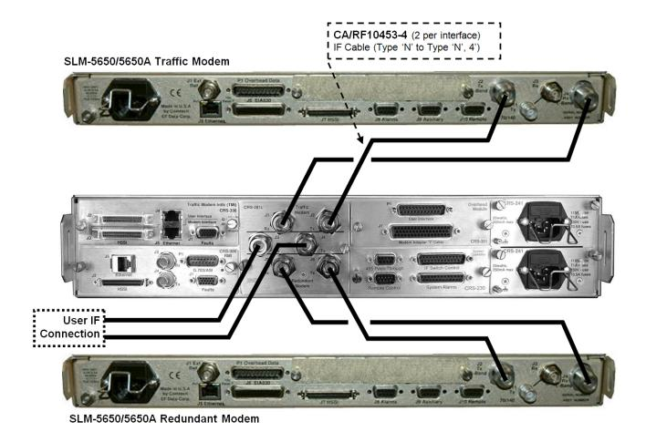
Figure 3-16. SLM-5650/5650A IF Cabling Example – CRS-281L (L-Band)
