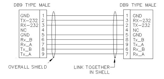
Figure A-7. RS-485 Null Modem Cable (CA/WR11419-1)
