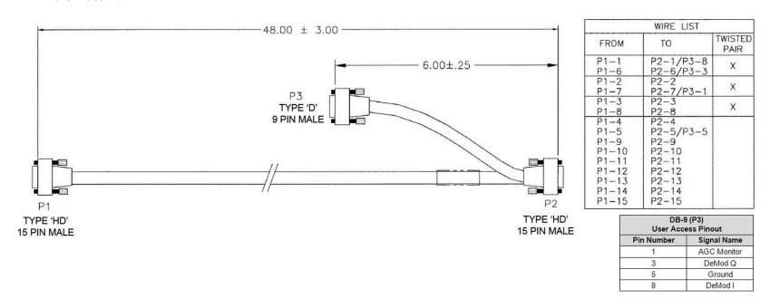
Figure A-11. SLM-5650/5650A Control 'Y' Cable (CA/WR12842-4)
