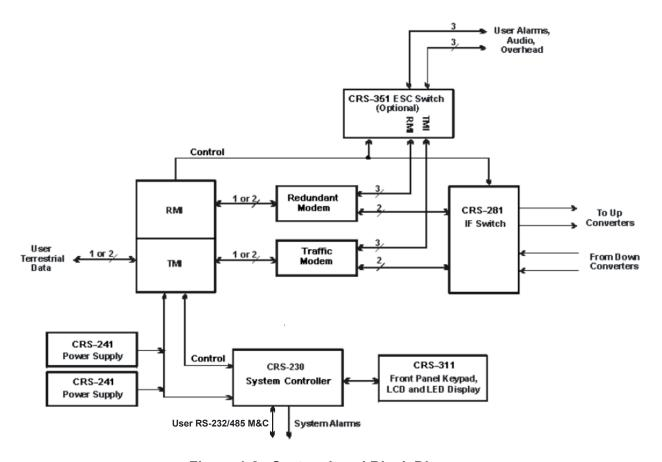
Figure 1-2. System-Level Block Diagram
