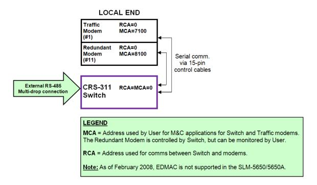
Figure B-2. CRS-311 Addressing Scheme Example: External RS-485 with SLM-5650/5650A Modems
