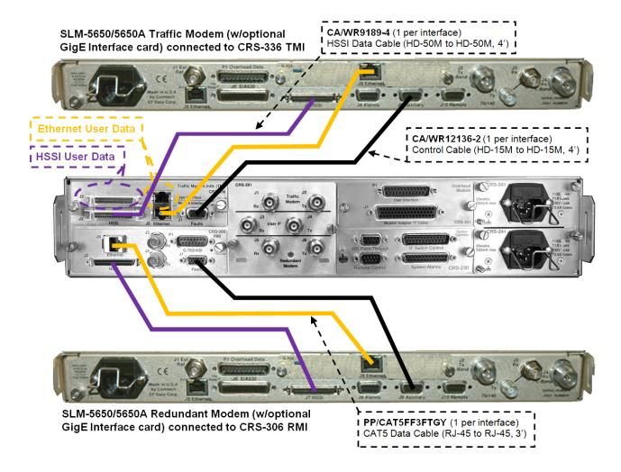
Figure 3-9. SLM-5650/5650A Control and HSSI, Ethernet Traffic (Single Port Bridge Mode)
