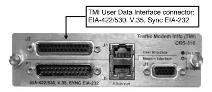
**Table 5-4** indicates the pinout for the DB-25F TMI User Data Interface connector (RS232/422/V.35): J2 on the CRS-316.
