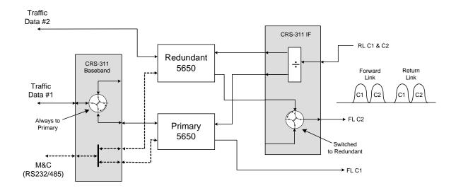
Figure D-2: CRS-311 in Independent Mode
