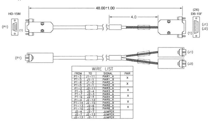
Figure A-8. Control 'Y' Cable for CDM-QxL with CnC® (CA-0000009)
