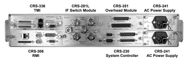
Figure 1-4. CRS-311 Rear Panel Configuration Example
