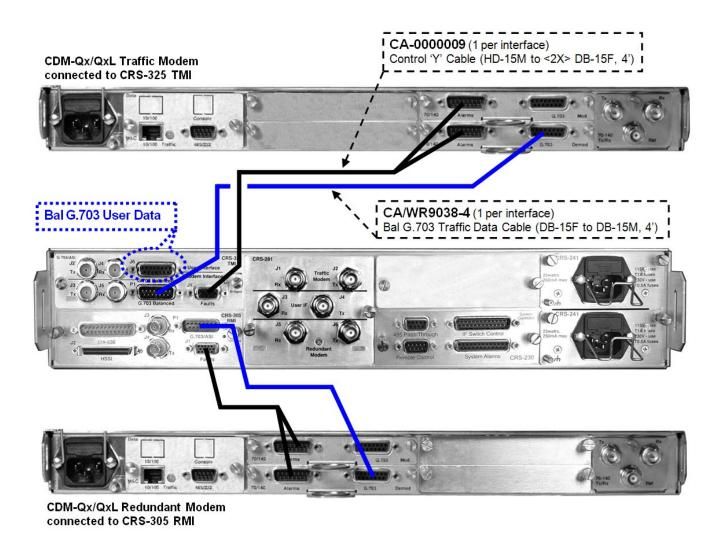
Figure 3-3. CDM-Qx/QxL Control 'Y' and Balanced G.703 Traffic Data Cables
