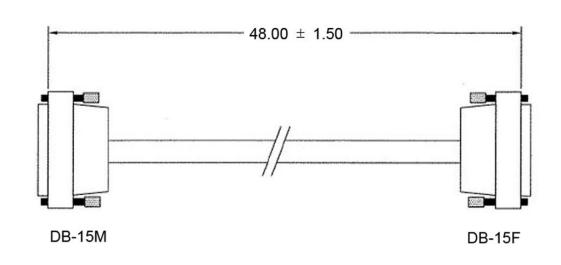
Figure A-13. Balanced G.703 Data Cable (CA/WR9038-4)
