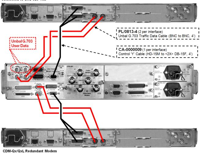
Figure 3-4. CDM-Qx/QxL Control 'Y' and Unbalanced G.703 Traffic Data Cables
