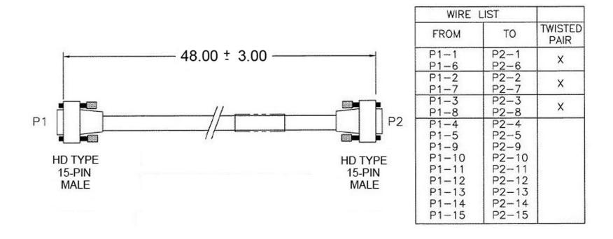
Figure A-9. SLM-5650/5650A Control Cable (CA/WR12136-2)
