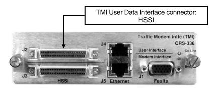
**Table 5-7** indicates the HD-50F Mini-D/SCSI-II HSSI User Data Interface connector: "J2" on the CRS-336 TMI.
