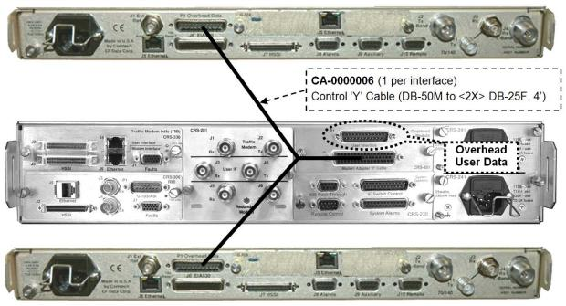
SLM-5650/5650A Redundant Modem connected to CRS-351
