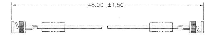
Figure A-14. Balanced G.703 / IF Cable, BNC 75 $\Omega$  (PL/0813-4)
