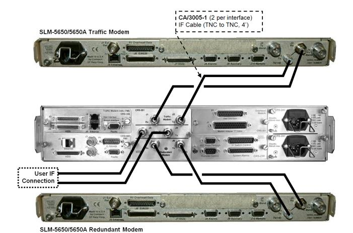
Figure 3-15. SLM-5650/5650A IF Cabling Example – CRS-281 (70/140 MHz)
