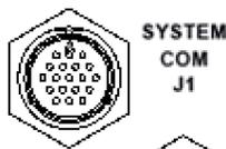
The **SYSTEM COM J1** connector is a 19-pin circular connector, type MS3112E14-19S. It serves as the primary input between the user and the PCCB for controlling and monitoring both SSPAs. Its pinout specification is provided in **Table 2-2**.
