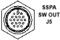
The **SSPA SW OUT J5** connector is a 19-pin circular connector, type MS3112E14-19S. It connects, via a “Y” cable, to the SSPA #1 and SSPA #2 waveguide switches. Its pinout specification is provided in **Table 2-4**.
