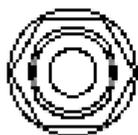
The **SSPA OUT J10** connector, located on the left side panel of the PCCB, is a Type ‘N’ female connector. It provides the RF signal output from the PCCB to SSPA #1.
