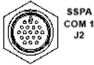
The **SSPA COM 1 J2** and **SSPA COM 2 J3** connectors are 19-pin circular connectors, type MS3112E14-19S. Each serves as the primary input/output interface between the PCCB and its specified SSPA. The typical pinout specification is provided in **Table 2-3**.
