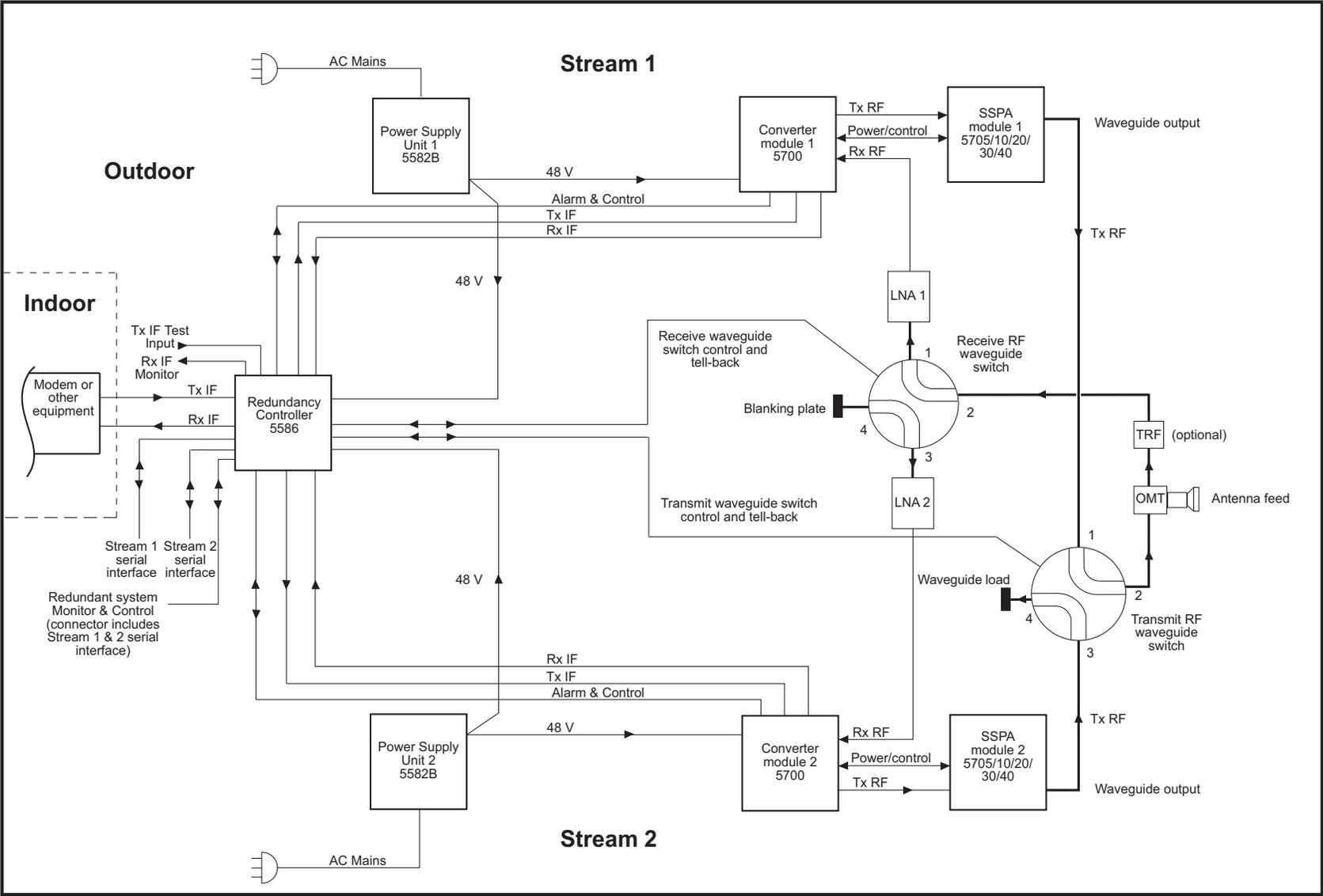
Figure 3-3: Block diagram of the dual switch redundancy system for the high power C-Band transceiver with separate waveguide switches
