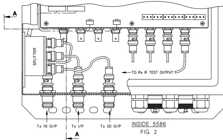
5586 Redundancy Controller
