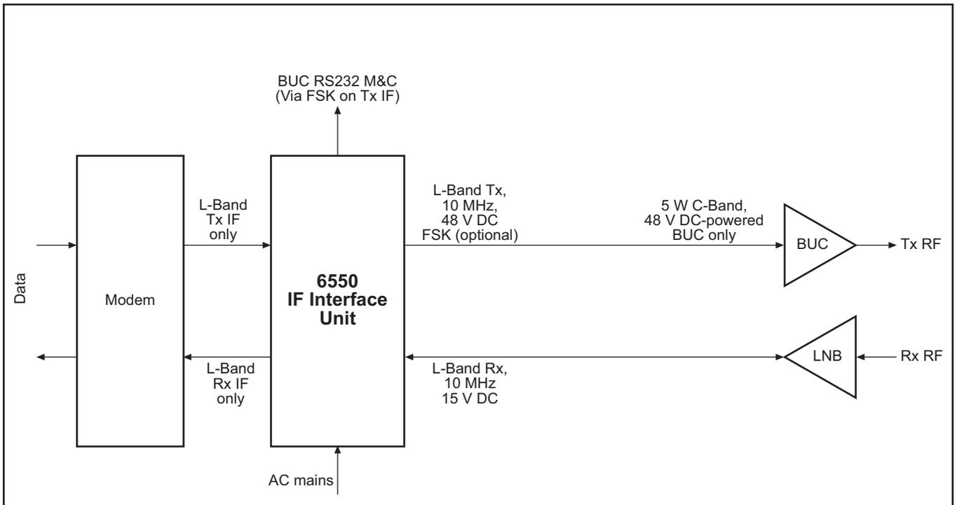
Figure 2: Typical configuration of a 6550 IF Interface Unit with a 6580B BUC Power Supply module
