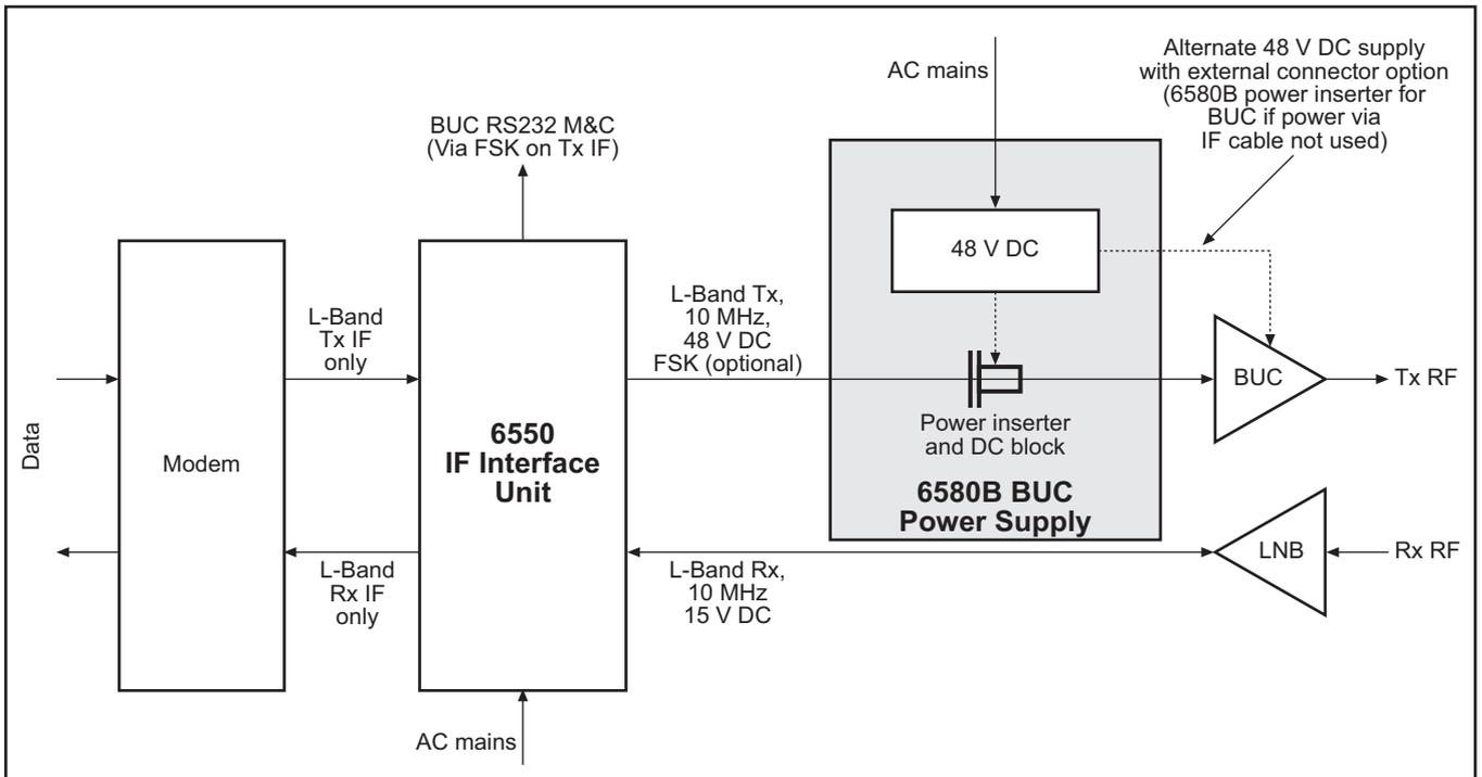
Figure 3: Typical configuration of a 6580B BUC Power Supply module
