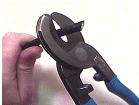
Figure B-1. Coax Cable Cutting Technique
