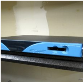
Upcom IRD+ HD Integrated Receiver Decoder Upcom IRD+ is a fully complete IRD with a complete list of options, including DVB-S/S2, ASI and IP Receiver, SD/HD MPEG-2 and H.264/MPEG-4 AVC Decoder Multiple Analog and Digital Outputs
