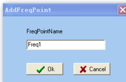
User can also click right mouse key to pop up the short-cut menu in device tree or in the left blank column, then the corresponding dialog box will pop up by choosing **Add Main Freq Point**. The device will confirm the given frequency while user clicks **OK**.
