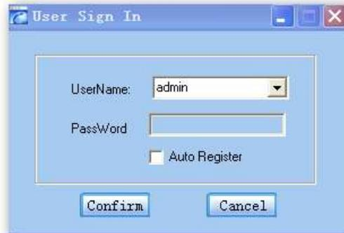
User can login the NMS by pressing **Confirm** key after inputting user name and password. Upon the inputs, the software will verify them with database record automatically. If both of them are correct, the main interface will appear. Both of the default user name and password are **admin**.
