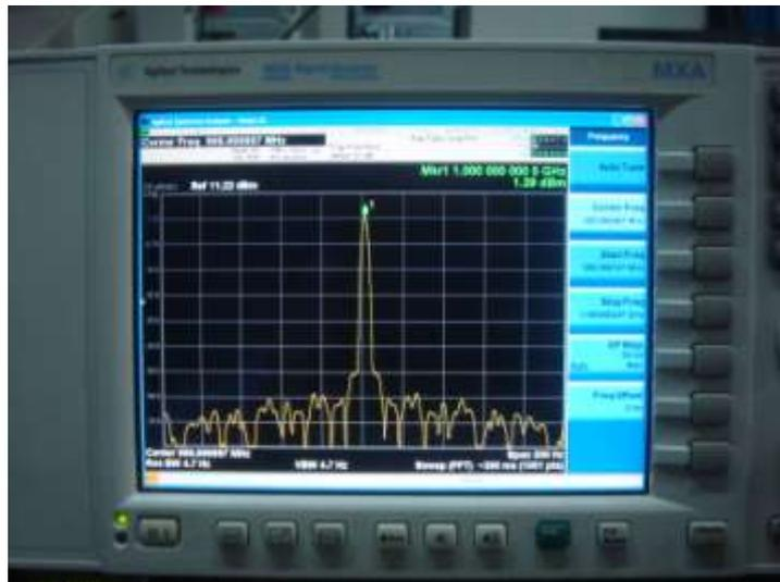
**Modulation:** The RF output carrier with modulation.
