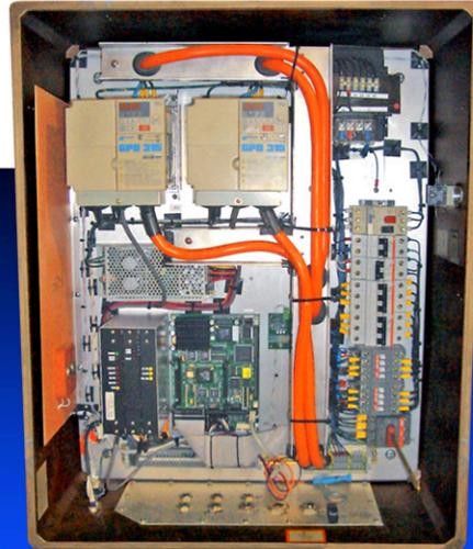
The ACS3000 controller provides three-axis control for antenna azimuth, elevation and feed polarization.
