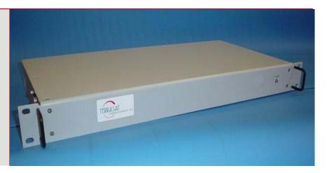
Terrasat's Indoor IBUC Power Supplies, models PSUI-1148 and PSUI-1248, run on AC mains power and provide 48 VDC power to the IBUC through a multi-conductor 16 AWG cable. The units are packaged in rack-mountable chassis with internal cooling fans.
