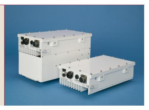
Terrasat's Outdoor BUC Power Supplies run on AC mains power and provide 24 or 48 VDC power to the IBUC through a multi-conductor 16 AWG cable. The unit is packaged in an environmentally protected outdoor enclosure. The form factor is compatible with Terrasat's universal mounting bracket.
