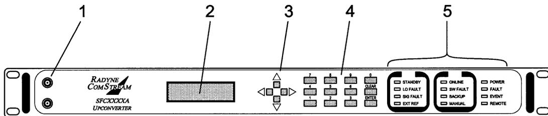
Figure 4-1. SFC Upconverters Front Panel Controls and Indicators
