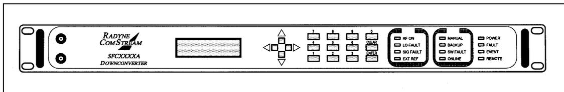
Figure 5-7. SFC Upconverter Front Panel with Monitor Ports
