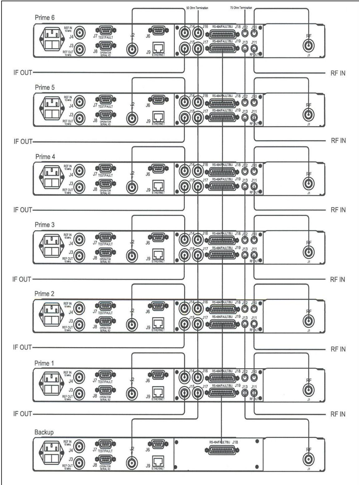
Figure 3-5. Chain Switching Operation in a 1:N Configuration.
