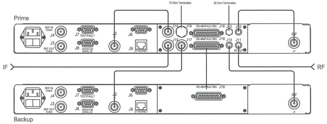
**Figure 3-4. Chain Switching Operation in a 1:1 Configuration**
