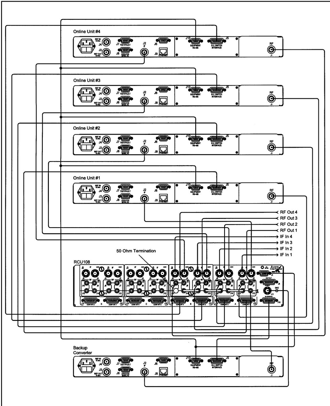
Figure 3-3. RCU108 Typical Interconnection with SFC Upconverters
