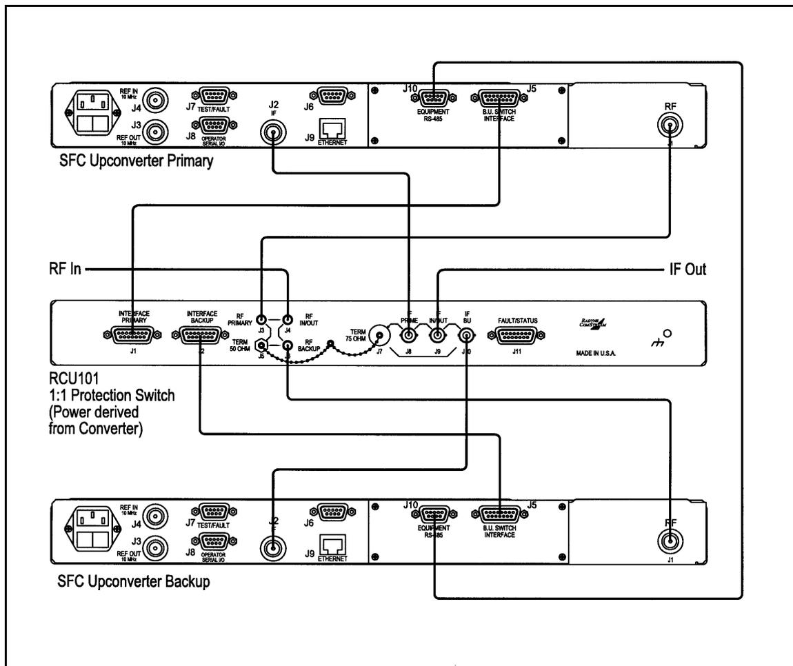
**Figure 3-2. RCU101 Typical Interconnection with SFC Upconverters**
