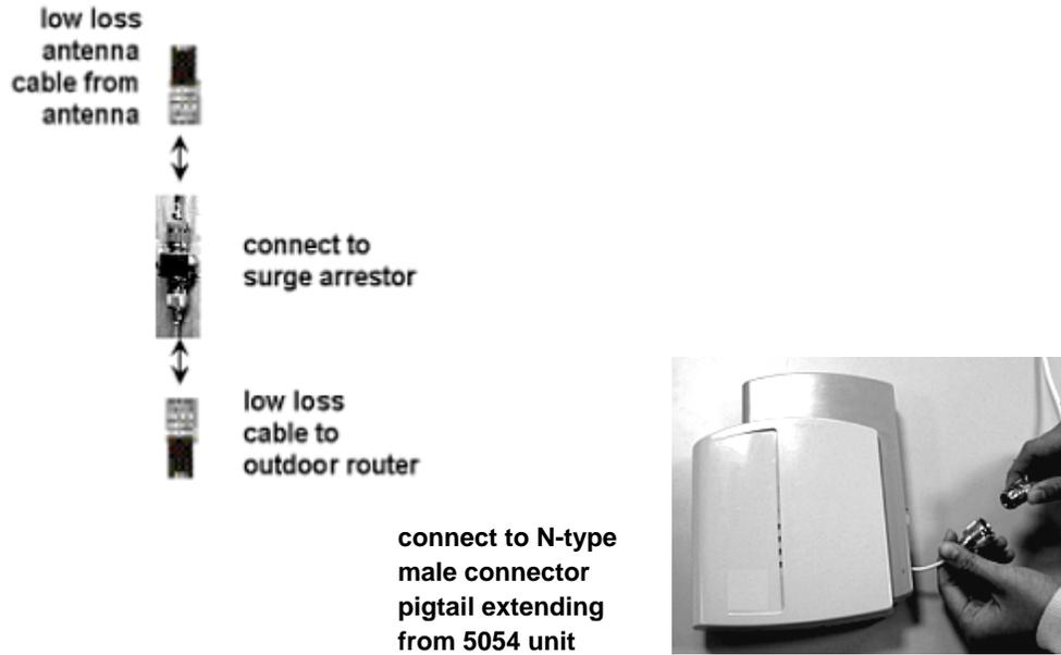
Figure 1. Cable Setup for 5054 Antenna Installation
