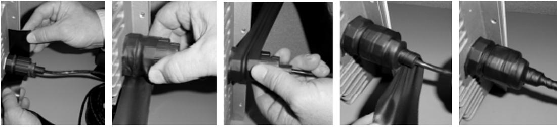
3. To protect the weatherproofing stretch tape from the effects of Ultra-Violet (UV) radiation (for example, from direct sunlight), you should protect the joint with two half-overlapped layers of any vinyl plastic electrical tape. Alternatively, you can apply silicone sealer to protect the weatherproofing tape from sunlight, rain and other weather conditions.
