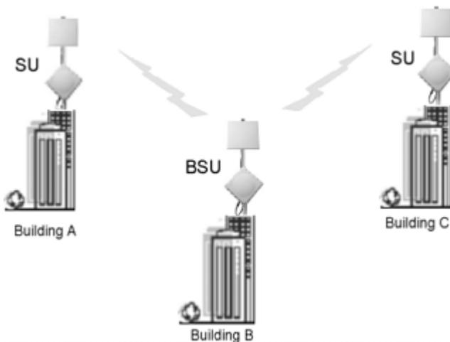
A link between two locations always consists of a Base Station Unit (BSU) and a Subscriber Unit (SU). A BSU can, depending upon its configuration, connect to one or more SUs; an SU, however, can connect to only one BSU.
