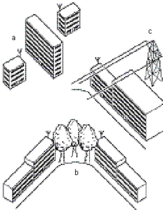
Figure 2. Potential Obstacles for a Directional Antenna
