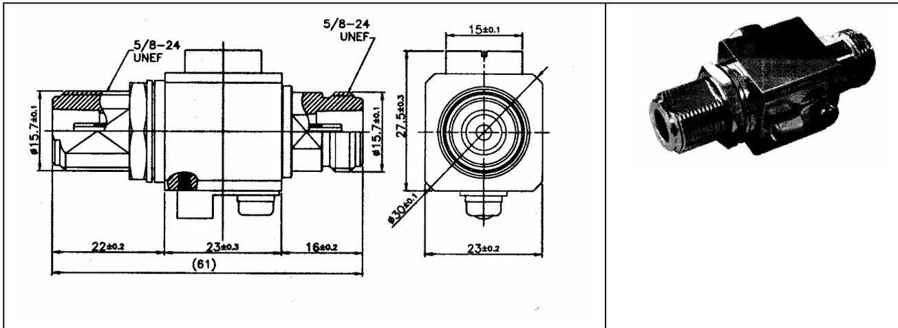
**CAUTION!** To avoid damage to electronic equipment and your radio equipment, always apply the surge arrester between the outdoor antenna installation and the radio hardware or other computing device that is connected to the outdoor antennas.
