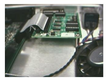
The HSSI card has three standoffs attached to the card. Also, notice that there are two ribbon cables attached to the HSSI. One of them is for connecting to the SNIP, if there is also a SNIP Ethernet option card installed.
