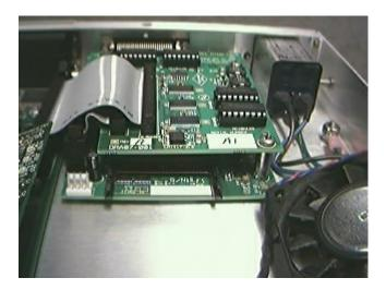
The Major difference is, you need to remove the two jackscrews holding the rear plate on the SNIP card. The new rear plate includes cutouts for both the HSSI and the SNIP.
