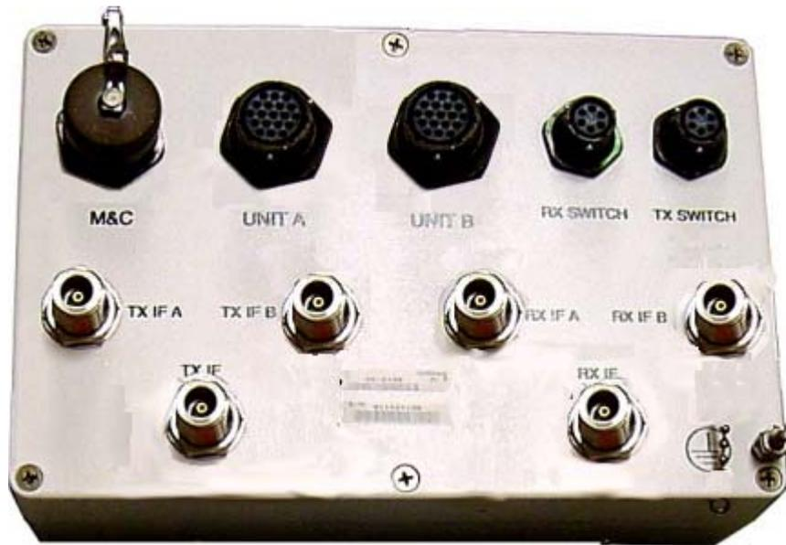
**Figure A-14. Assembly, TX/Remote Switch, AS/0490**
