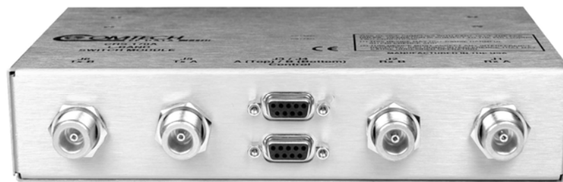
J6 TX B J5 TX A J3 Control A J2 RX B J1 RX A J4 Control B
