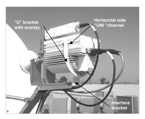
Figure C-7. SSPA Installed
