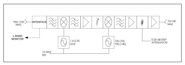
Figure 3-13. L-Band to IF Down Converter Block Diagram
