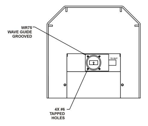
Figure 2-6. Output Connection for the 16 Watt SSPA (Waveguide)
