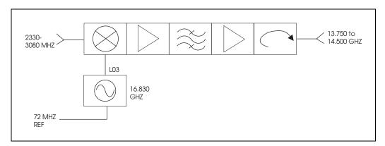
Figure 3-11. S to Ku-Band Up Converter Module
