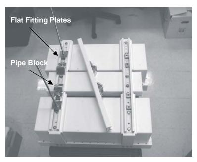
Figure D-3. KST-2000A 1:1 Converters With Mounting Brackets
