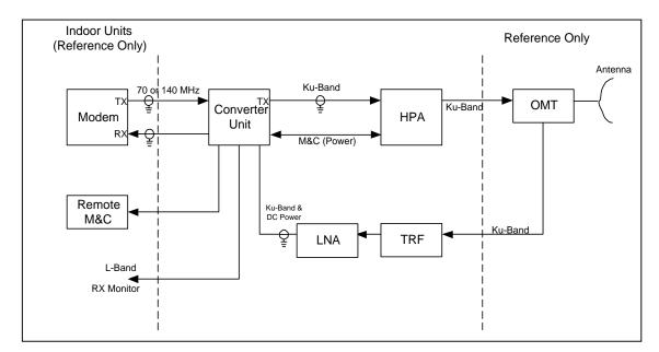
Figure 1-3. Single Thread KST-2000A System
