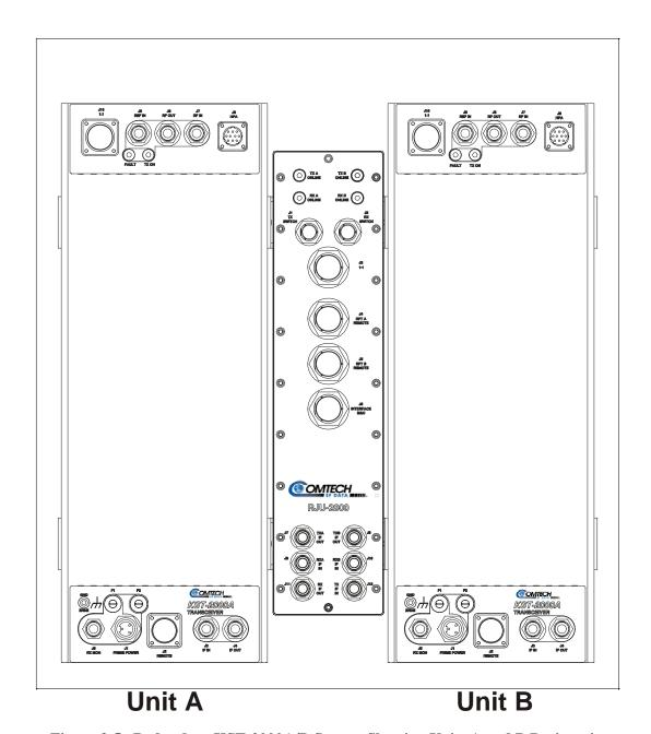
Figure 3-5. Redundant KST-2000A/B System Showing Units A and B Designation
