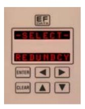
Figure 5-11. Redundancy Menu
