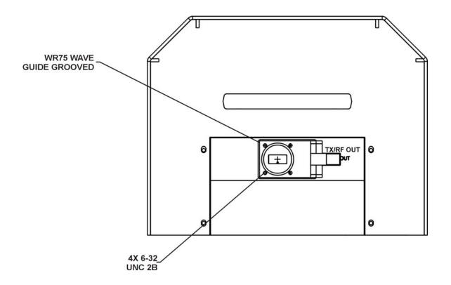
Figure 2-9. Output Connection for the 25/32/40 Watt SSPA (Waveguide)
