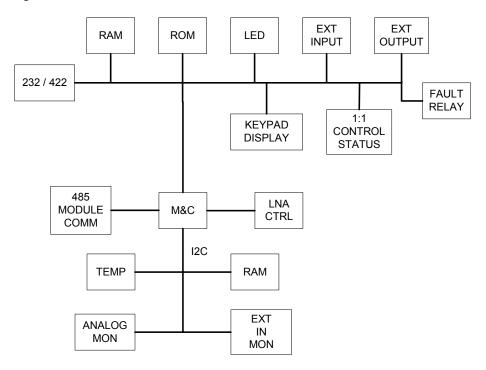
Figure 3-9. Monitor and Control (M&C) Block Diagram
