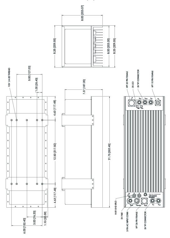
Figure A-6. KST-2000A/B Converter Equipment Outline
