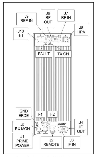
Figure 2-1. I/O View of KST-2000A/B Converter Unit
