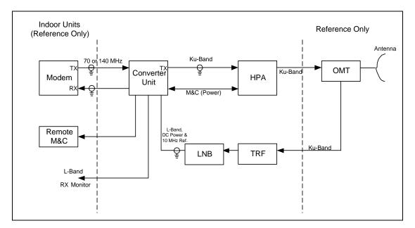
Figure 1-4. Single Thread KST-2000B Block Diagram
