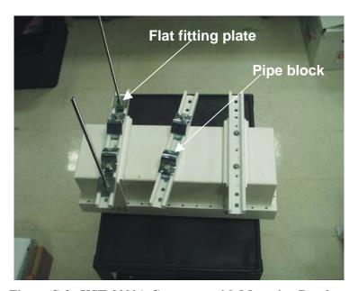
Figure C-3. KST-2000A Converter with Mounting Brackets
