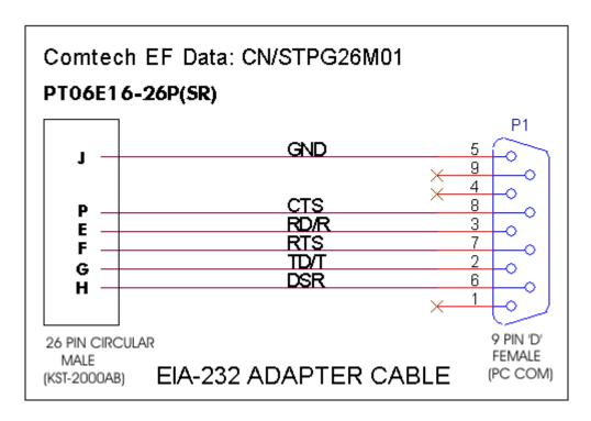
Figure 2-3. Serial (EIA-232) Adapter Cable Wiring Diagram
