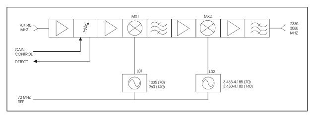
Figure 3-10. IF to S-Band Converter Module Block Diagram
