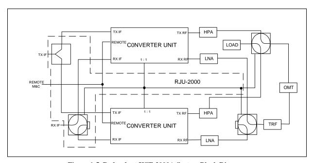
Figure 1-5. Redundant KST-2000A System Block Diagram
