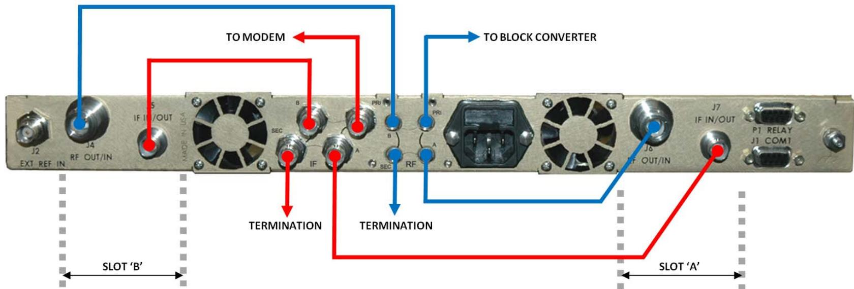
Figure C-2. LBC-4000 Redundancy Cabling Requirements
