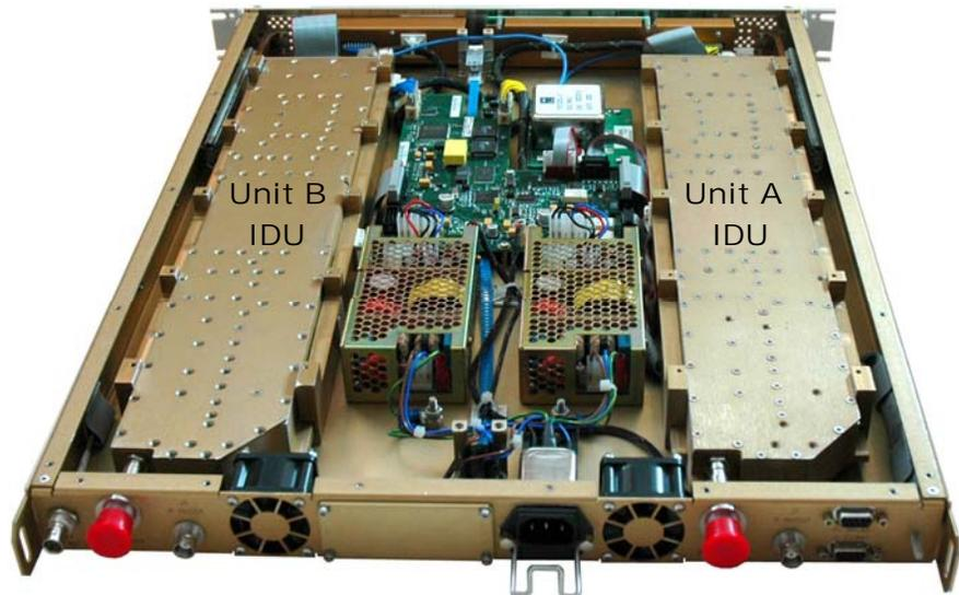
**Figure B-1. LBC-4000 Chassis – IDU Modules**
