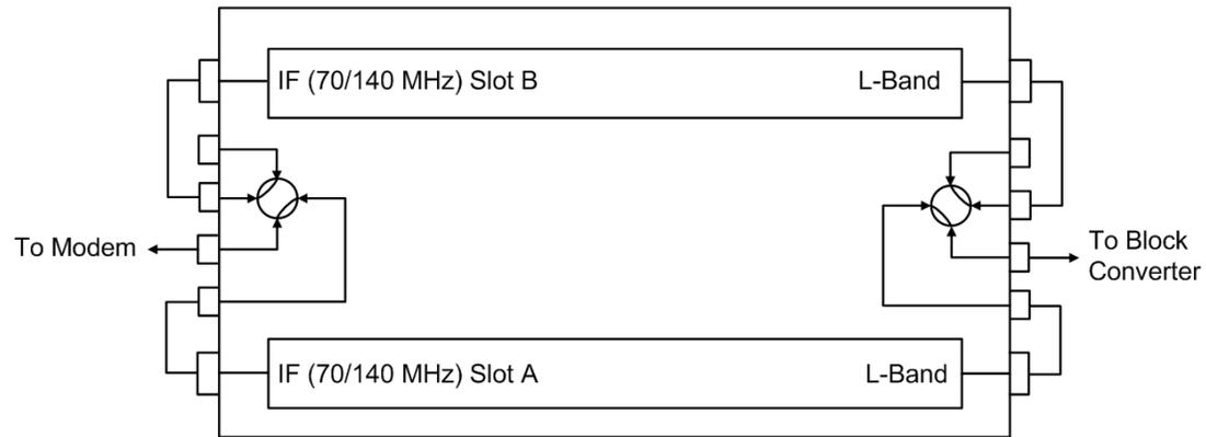
Figure C-1. LBC-4000 Redundancy – Functional Schematic
