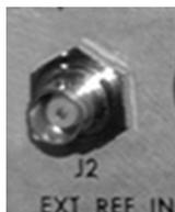
The **J2 External Reference Input** is used to supply a master reference to the entire chassis. The input signal supplied here by the user is used for phase-locking the internal 10MHz reference oscillator to a customer-provided 5 or 10 MHz station clock. The impedance is matched for 50/75Ω, and requires a level in the range 0.5V-4.0Vpp square or sine wave.
