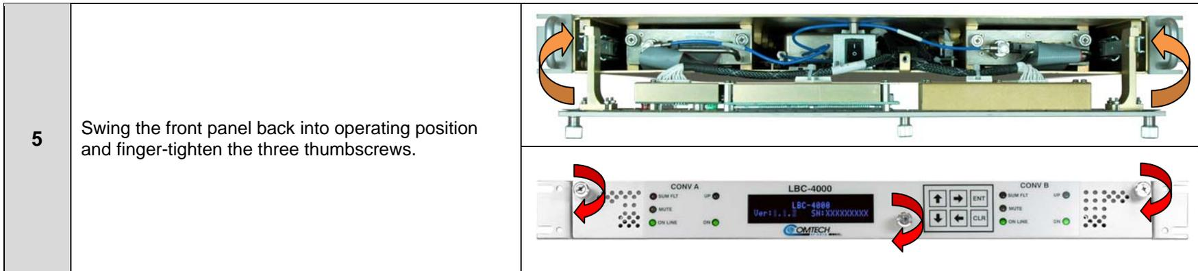
The IDU module installation has been completed and the LBC-4000 L-Band Up/Down Converter System is ready to be connected to other equipment. Refer to **Chapter 3. REAR PANEL CONNECTIONS** for further information.
