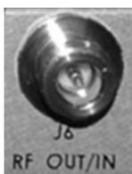
The **J6 RF OUT/IN** connector is a Type 'N' female connector that provides either an L-Band output signal interface (with the Downconverter IDU installed), or an L-Band input signal interface (with the Upconverter IDU installed).
