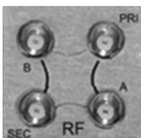
The **RF Primary A / Secondary B** connector pairs are Type 'SMA' female connectors that provide the RF “baseball” switch for optional redundant operations. Refer to **Figure C-2** in **Appendix C. LBC-4000 REDUNDANCY OPERATION** for interconnection between these connectors to others located on the LBC-4000 rear panel and on other external equipment.
