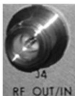
The **J4 RF OUT/IN** connector is a Type 'N' female connector that provides either an L-Band output signal interface (with the Downconverter IDU installed), or an L-Band input signal interface (with the Upconverter IDU installed).
