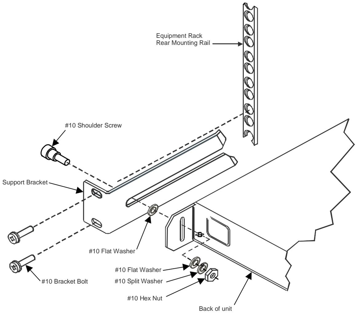
**Figure 2-3. Optional Rear-Mounting Support Bracket Kit Installation**
