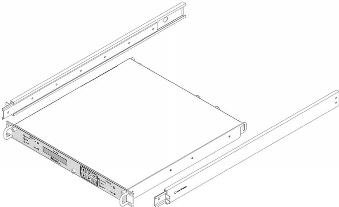
**Figure 2-2. LBC-4000 Optional Side-Railings Installation (FP/SL0006)**
