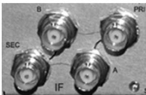
The **IF Primary A / Secondary B** connector pairs are Type 'BNC' female connectors that provide the IF “baseball” switch for optional redundant operations. Refer to **Figure C-2** in **Appendix C. LBC-4000 REDUNDANCY OPERATION** for interconnection between these connectors to others located on the LBC-4000 rear panel and on other external equipment.
