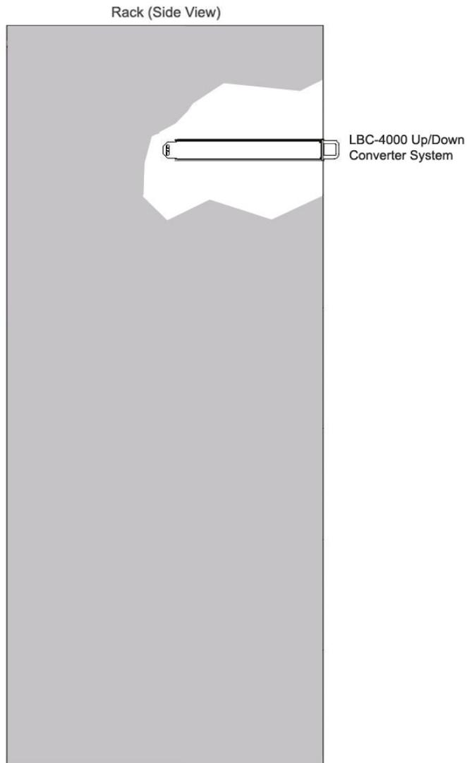
**Figure 2-1. LBC-4000 Standard Rack Cabinet Installation**
