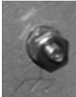
A #10-32 stud is used for connecting a common chassis ground among equipment.
