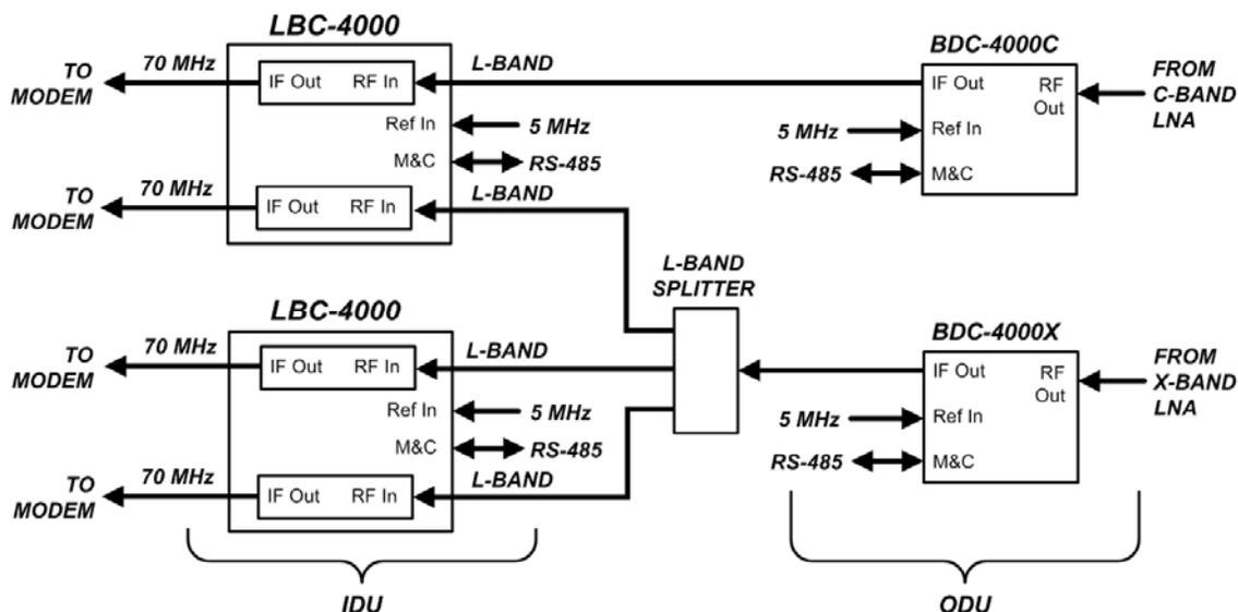
**Figure 1-2. LBC-4000 Typical Application Block Diagram**
