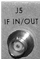
The **J5 IF IN/OUT** connector is a Type 'BNC' female connector that provides either a downconverted IF input signal (with the Downconverter IDU installed), or an upconverted IF output signal (with the Upconverter IDU installed).
