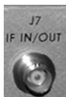
The **J7 IF IN/OUT** connector is a Type 'BNC' female connector that provides either a downconverted IF input signal (with the Downconverter IDU installed), or an upconverted IF output signal (with the Upconverter IDU installed).
