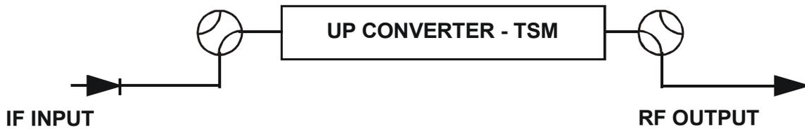
Figure 8. Non-Redundant Converter Configuration With Transmit Switch Module (TSM-XX) Installed
