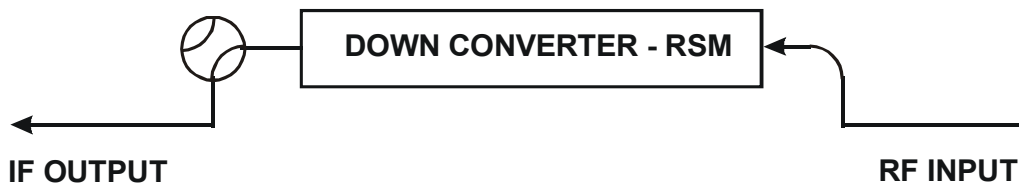
Figure 8. Non-Redundant Converter Configuration With Receive Switch Module (RSM-XX) Installed
