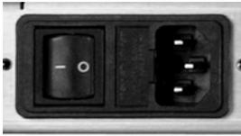
The IEC line input connector contains the ON/OFF switch for the unit. It is also fitted with two fuses, one each for line and neutral connections (or L1, L2, where appropriate). These are contained within the body of the connector, behind a small plastic flap.
