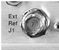
The **J1 External Reference Input** is used to supply a master reference to entire chassis. Use of an external reference is not required. The input/output signal supplied here by the user is used for phase-locking the internal 10MHz reference oscillator, and can be 1, 2, 5, or 10 MHz. The impedance is matched for 50/75Ω, and requires a level in the range 0.5V-4.0Vpp square or sine wave.
