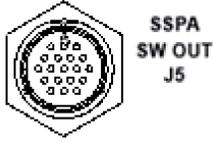
The **SSPA SW OUT J5** connector is a 19-pin circular connector, type MS3112E14-19S. It connects, via a “Y” cable, to the SSPA #1 and SSPA #2 waveguide switches. Its pinout specification is provided in **Mating connector:** ITT Cannon MS3116J14-19P
