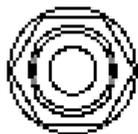
The **SSPA OUT J10** connector, located on the left side panel of the PCCB, is a Type ‘N’ female connector. It provides the RF signal output from the PCCB to SSPA #1.
