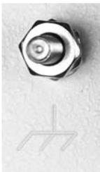
A #10-32 stud is provided on the front panel of the PCCB for connecting a common chassis ground among equipment.
