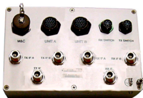
Figure C-12. Remote Switch Box Assembly, AS/0490
