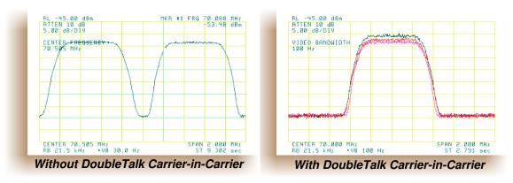
Figure 3: DoubleTalk™ Carrier-in-Carrier™ Transponder Spectrum
