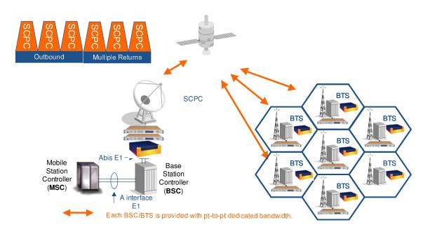
Figure 4: The Point-to-point topology with the Memotec bandwidth optimization.
