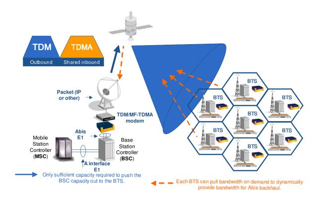
Figure 6: Point-to-multipoint TDM/MF-TDMA solution
