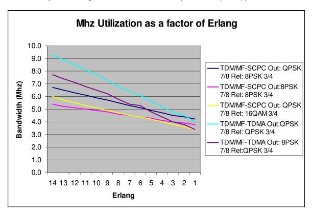
Figure 7: MHz usage as a factor of Erlang.
