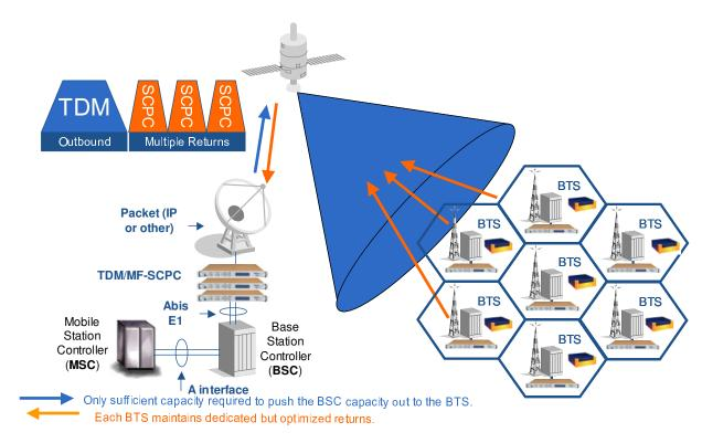
Figure 5: Point-to-multipoint TDM/MF-SCPC solution (AbisXtender)
