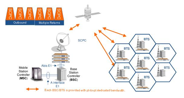
Figure 2: The Point-to-point SCPC topology.
