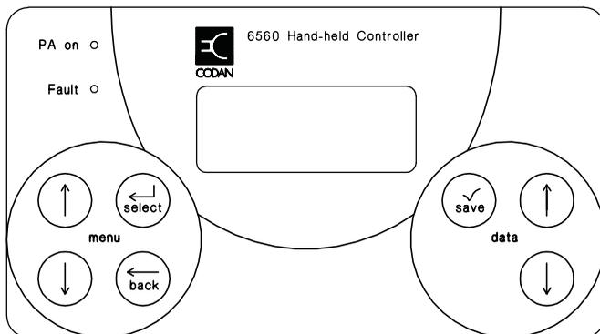
Figure 2: The front panel of the remote controller
