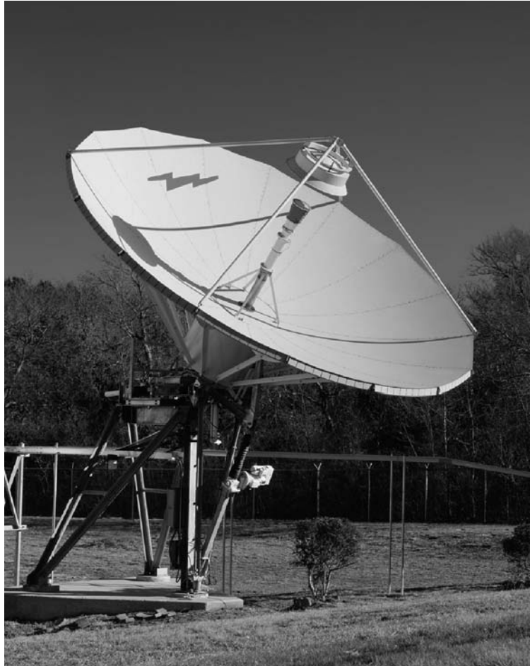
7.3-Meter Earth Station Antenna
